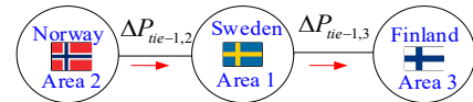
Fig. 4. Simplified model of the NPS. \Delta P_{tie} is used to represent the incremental active power change during a system frequency event
