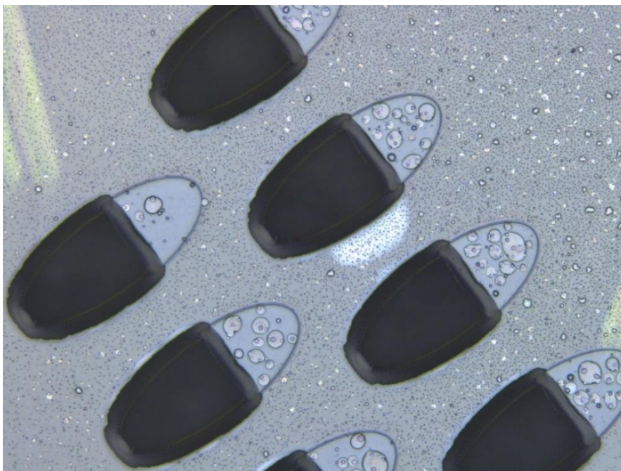
Figure 5-21 the structure of the wafer was observed after the deep dry silicon etching . The image was taken by Leica microscope in bright field mode and 5X magnification
