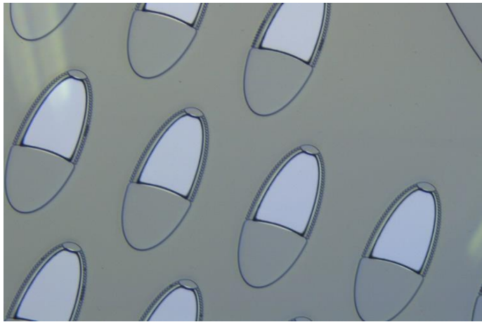
Figure 5-13 shows the pillar structure and substrate structure between the pillars. The image was taken by Leica Optical microscope with bright field mode and 5X magnification
