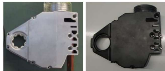
Fig. 12. Metallic crankcase functioning as heat sink with surface area about twice the size of the current path of the LBS.
