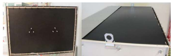
Fig. 5. Switchgear enclosure surfaces painted with matt finish black paint. Back surface (left) and top surface (right).
