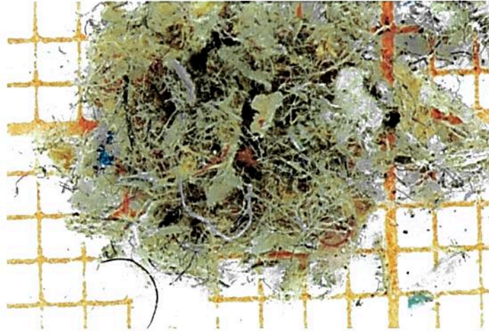
Figure A.3: Structure of a RDF sample from the variographic experiments at Brevik Norcem.
