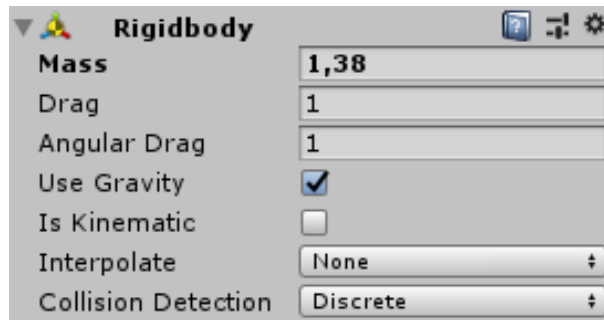
FIGURE 4.4: Unity rigidbody type with mass, and both drag and angular drag for air friction.
