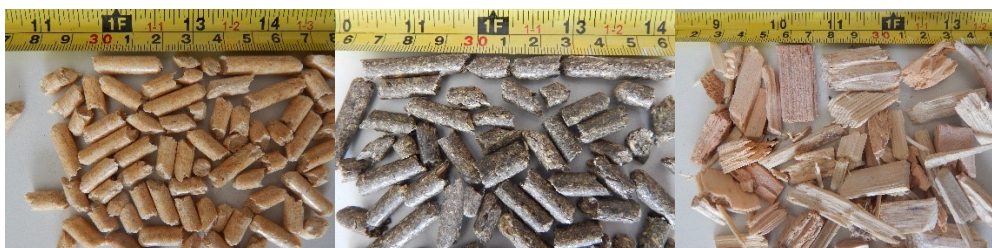
Figure 4: Gasifier feed material and size scales, wood pellets, grass pellets and wood chips (from left to right)
