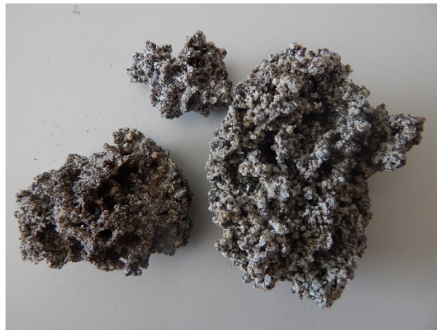
Figure 15: Formation of agglomerates during grass pellet gasification
