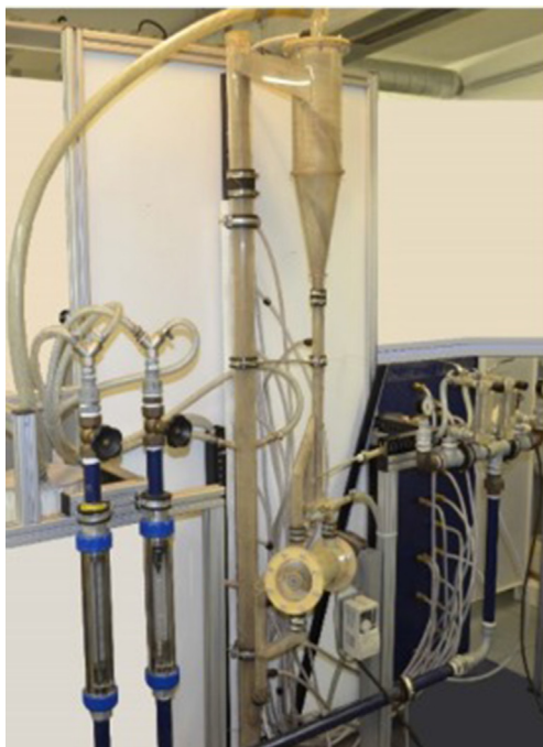
Fig. 3. Circulating fluidized bed experimental rig (Thapa et al., 2016).
