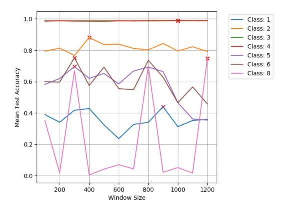
FIGURE 5.1: Grid search results of the window size, showing mean test accuracy for each fault and their respective window sizes.
