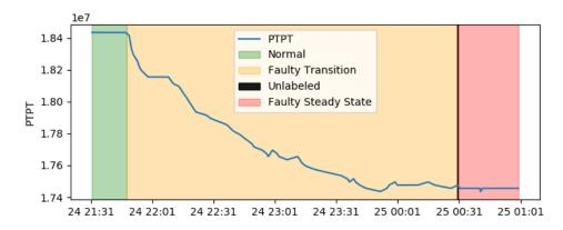
FIGURE 3.3: Real instance of 'Abrupt increase of BS&W' showing pressure at TPT.
