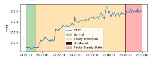
FIGURE 3.4: Real instance of 'Abrupt increase of BS&W' showing temperature at TPT.
