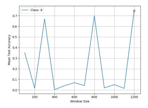
FIGURE A.7: Grid search result showing mean test accuracy for the different window sizes for fault 8.
