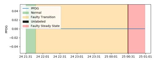
FIGURE 3.5: Real instance of 'Abrupt increase of BS&W' showing pressure at PDG.
