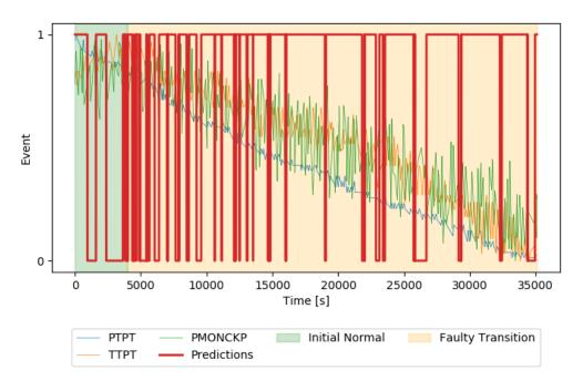
FIGURE 5.9: Example of a real instance of Class 5 along with the rapid inconsistent system classifications. Event values '1' and '0' denote normal and faulty states
