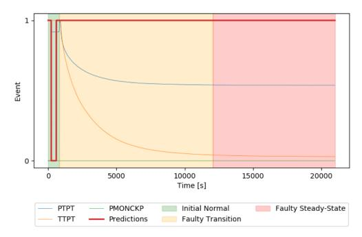
FIGURE 5.5: Example of a real instance of Class 2 along with the system classification, where the system achieved below than 90% accuracy on initial normal. Event values '1' and '0' denote normal and faulty states.
