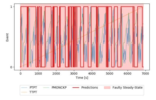
FIGURE 5.2: Example of a real instance of Class 4 showing the inconsistency of the system classification, where only 70% of the samples were correctly classified. Event values '1' and '0' denote normal and faulty states.
