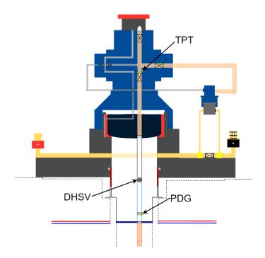
FIGURE 3.2: Simplified schematic of a typical subsea Christmas tree based on [32].
