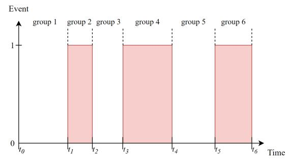
FIGURE 4.6: Illustration of how the samples are categorized into groups based on the condition of the event. These groups are used when applying the Group k-fold strategy during training.
