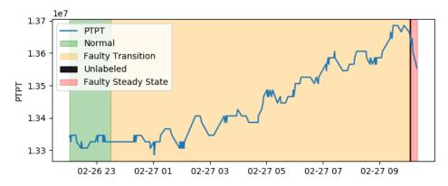
FIGURE 3.7: Real instance of 'Scaling in PCK' with sensor variable P-TPT.
