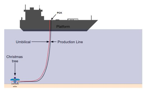
FIGURE 3.1: Simplified schematic of a typical offshore naturally flowing well based on [32].
