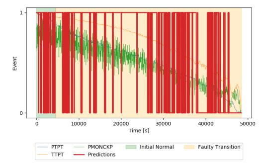
FIGURE 5.8: Example of a real instance of Class 5 along with the rapid inconsistent system classifications. Event values '1' and '0' denote normal and faulty states.
