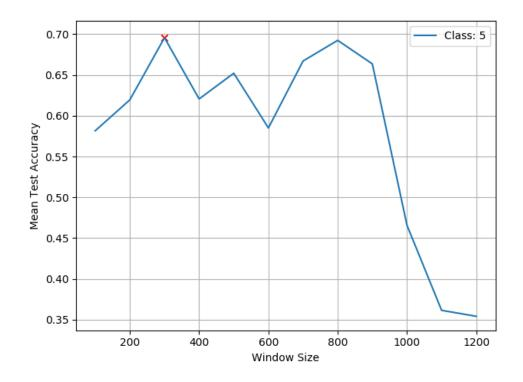
FIGURE A.5: Grid search result showing mean test accuracy for the different window sizes for fault 5.
