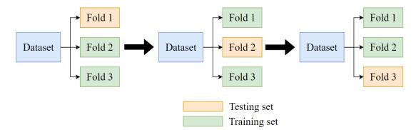
FIGURE 4.5: Illustration of the k-fold strategy. The dataset is split into k subsets, where each iteration uses the orange fold as a test set to evaluate the model and the remaining green folds are used to train the model. This process is repeated until each orange fold of all k folds have been used as a testing set to evaluate the model.
