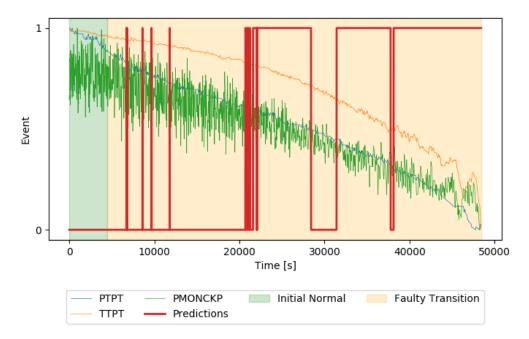
FIGURE 5.3: Example of a real instance of Class 5 showing the inconsistency of the system classification, where only 54% of the samples were correctly classified. Event values '1' and '0' denote normal and faulty states.
