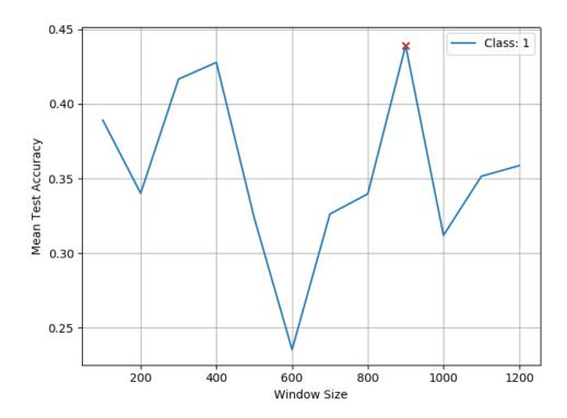
FIGURE A.1: Grid search result showing mean test accuracy for the different window sizes for fault 1.
