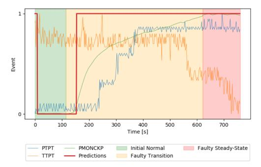
FIGURE 5.10: Example of a real instance of Class 6 along with the system classification, where the system achieved below than 90% accuracy on initial normal. Event values '1' and '0' denote normal and faulty states.
