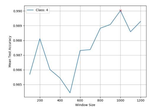
FIGURE A.4: Grid search result showing mean test accuracy for the different window sizes for fault 4.
