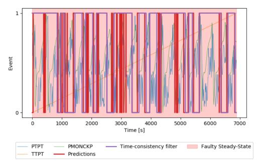
FIGURE 5.11: Example of a real instance of Class 4 along with the rapid inconsistent system classifications and with the time-consistency filter. Event values '1' and '0' denote normal and faulty states.
