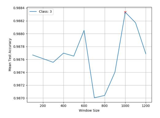
FIGURE A.3: Grid search result showing mean test accuracy for the different window sizes for fault 3.
