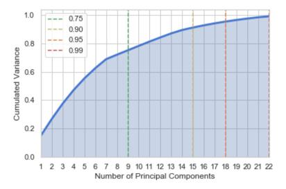
FIGURE 4.3: Principal component analysis performed on the training set of the 3W dataset. In this case, the data had a total of 72 features, which were extracted from the computation of nine statistical features.
