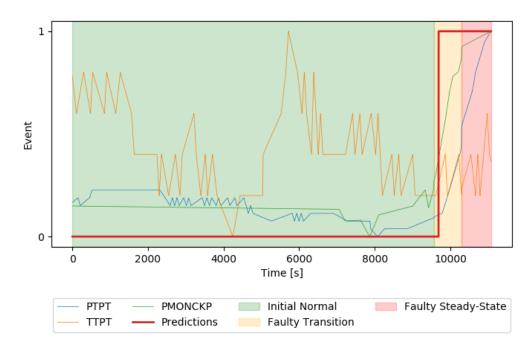
FIGURE 5.6: Example of a real instance of Class 6 along with the system classification. All samples belonging to initial normal and steady-state were correctly classified. However, the transient state only accomplished 80% accuracy. Event values '1' and '0' denote normal and faulty states.
