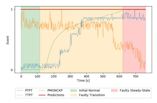
FIGURE 5.4: Example of a real instance of Class 6 along with the system classification, where the system was not able to correctly classify a single sample in the initial normal state. Event values '1' and '0' denote normal and faulty states.
