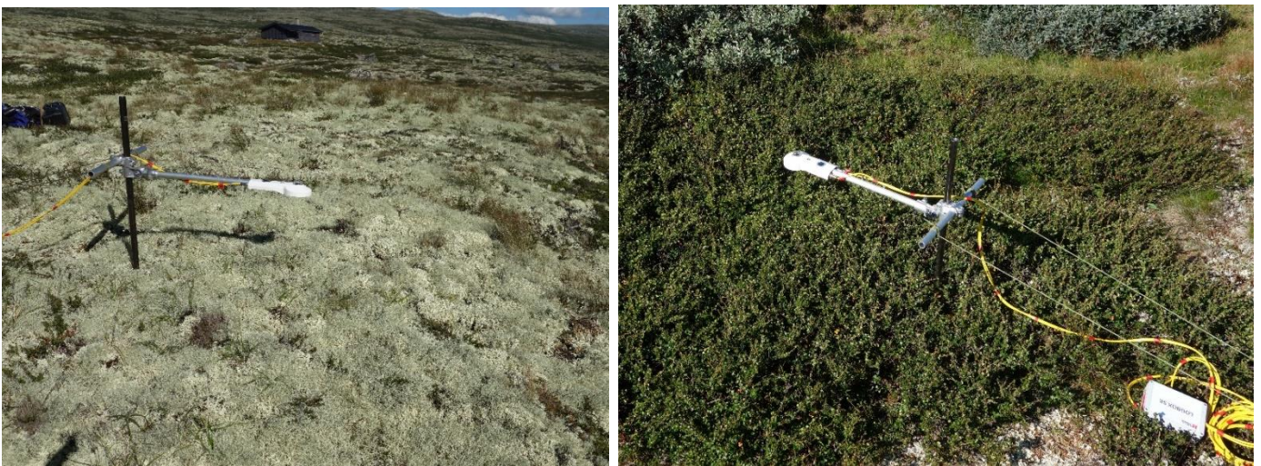
Figure 4: Setup for albedo measurements at one lichen plot (left) and one shrub plot (right)
