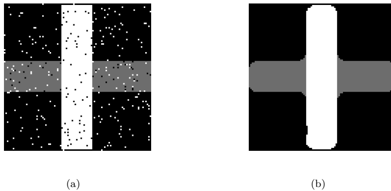
Figure 2.2: Median filter (a) grayscale image degraded by salt and pepper noise; (b) filtered image with [9 \times 9] kernel size median filter.
