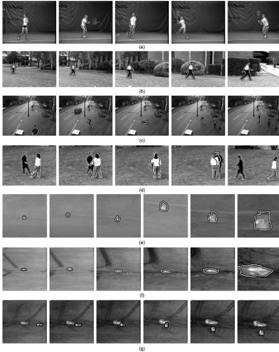
Figure 2.20: A snippet from Yilmaz et al. (2004) showing the contour based tracking of various objects.
