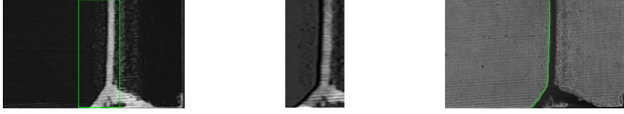
Fig. 6. Template matching process left: a filtered image from CO_2 experiment with a bounding box for matching, center : MSE calculated from matching within the bounding box, right: the result of choosing the minimum MSE in each row presented by the green curve in a raw image of the same image in left.
