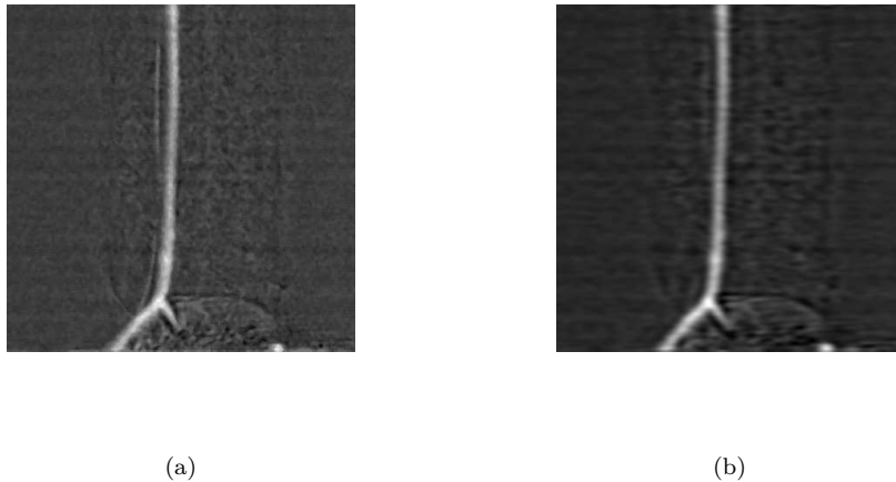
Figure 4.1: Image filtering (a) median filtering corresponding to top right image from Figure 1.8 with [9 \times 9] kernel size. (b) Frequency filtering corresponding to Figure 3.6 with cut off of 50 Hz.
