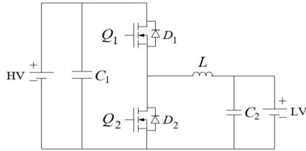
Figure 3.9: Buck-boost bidirectional DC-DC converter [42].
