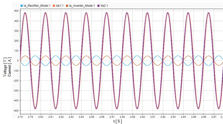
Figure 5.29: AC voltage and current for rectifier and inverter mode in phase A.
