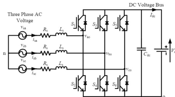
Figure 3.3: Three-phase two-level H-bridge bidirectional three-phase AC-DC converter [38].
