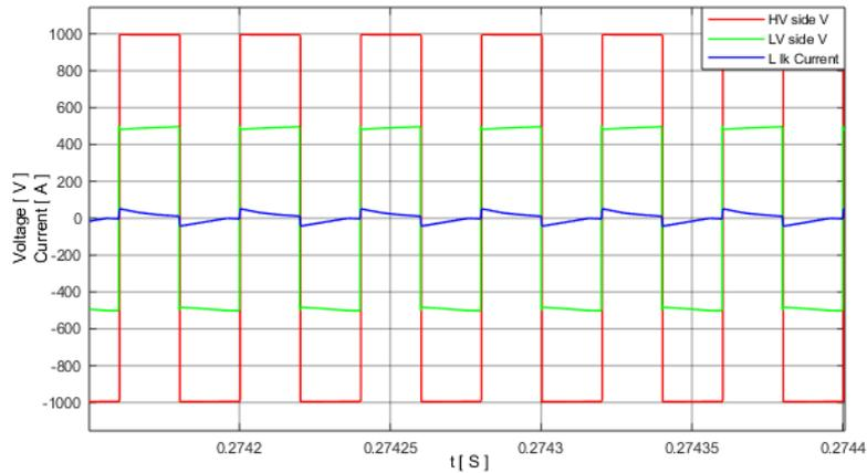
Figure 6.14: HV and LV side voltages and inductor current displaying soft switching.
