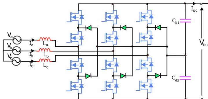
Figure 3.5: Three-phase three-level neutral point clamp AC-DC converter [30].
