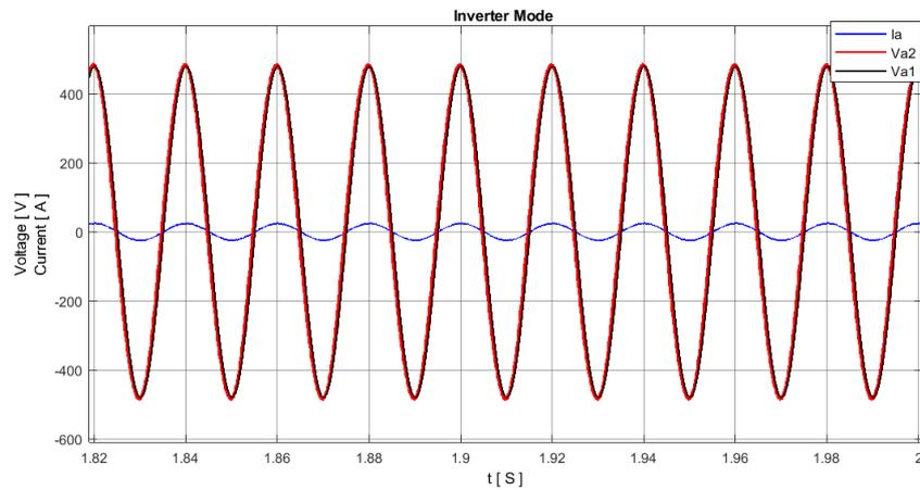
Figure 5.22: AC voltage generated by the inverter, AC grid voltage, and current (25 A).
