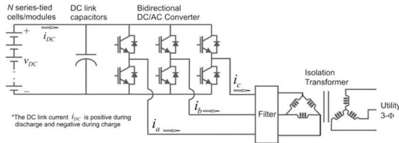
Figure 3.6: Single-stage three-phase bidirectional AC-DC converter [10].
