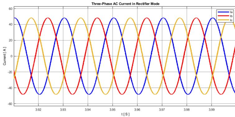
Figure 5.15: Three-phase grid currents during charging.
