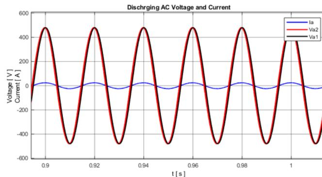
Figure 6.13: AC voltage and current when power transfer to the grid.
