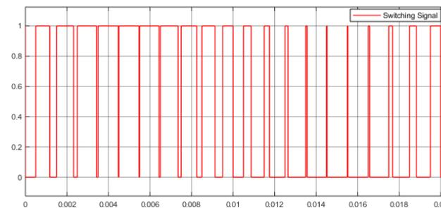
Figure 5.12: Generated gate pulse switching.
