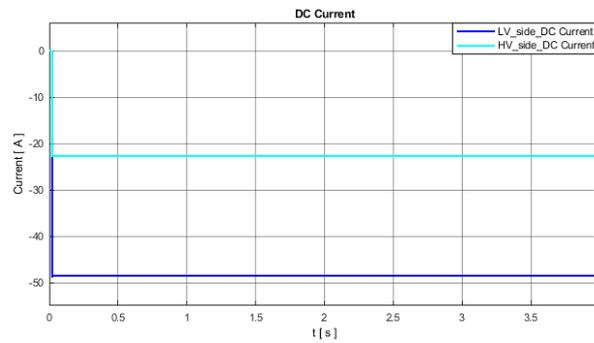
Figure 6.4: Average charging DC current in the LV and HV side  $\varphi = 2.16^\circ$ .
