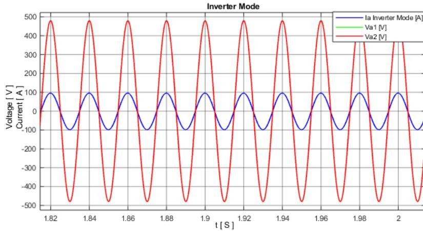
Figure 5.6: AC voltage and current under inverter mode with a  $2^\circ$  phase angle.
