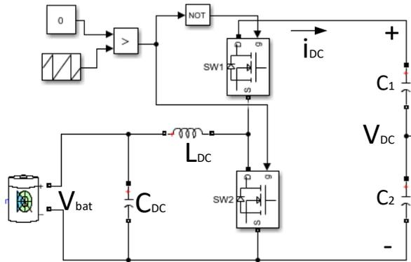
Figure 5.8: Bidirectional DC-DC converter.
