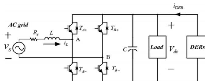
Figure 3.1: A bidirectional single-phase ac-dc converter in a load connected to dc microgrid and the grid [34]
