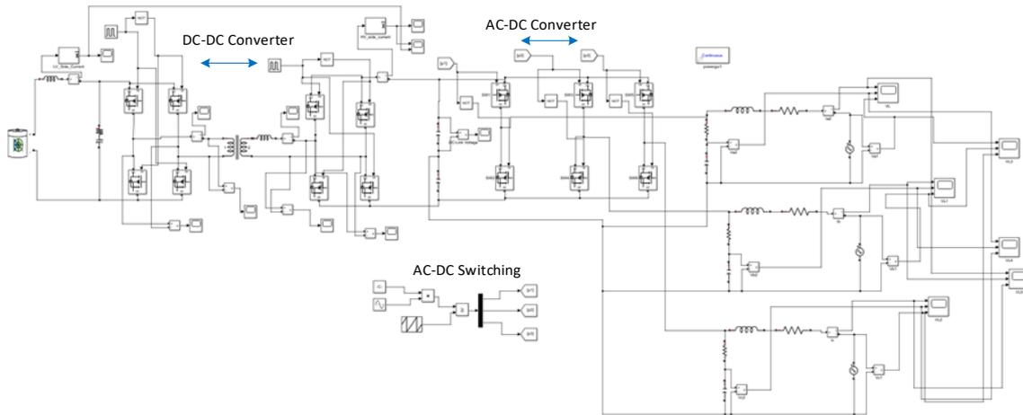
Figure 6.15: Simulation model proposed for EV charger with galvanic isolation.
