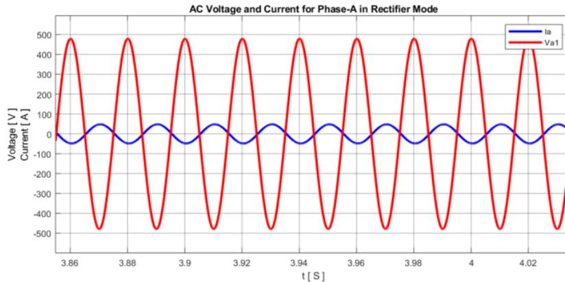
Figure 5.13: AC side voltage and current in phase A during charging.
