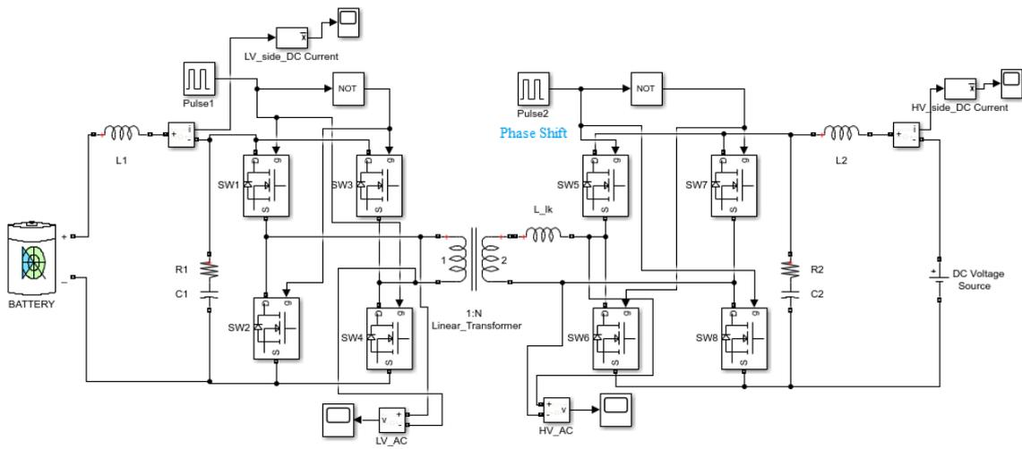
Figure 6.1: Bidirectional dual active bridge DC-DC converter.
