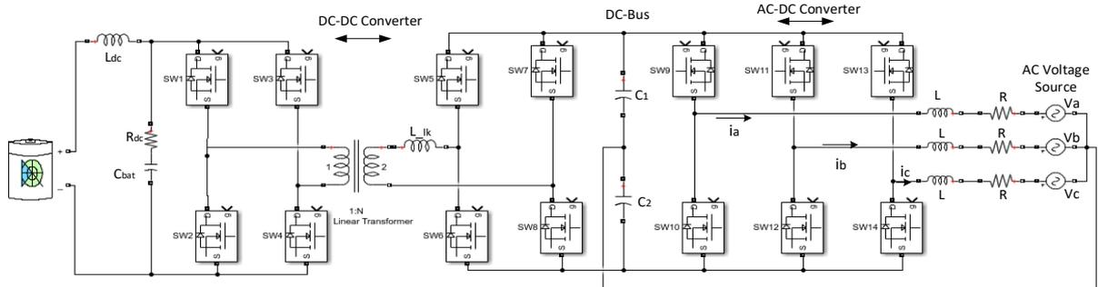
Figure 6.7: A two-stage bidirectional EV charger with galvanic isolation.
