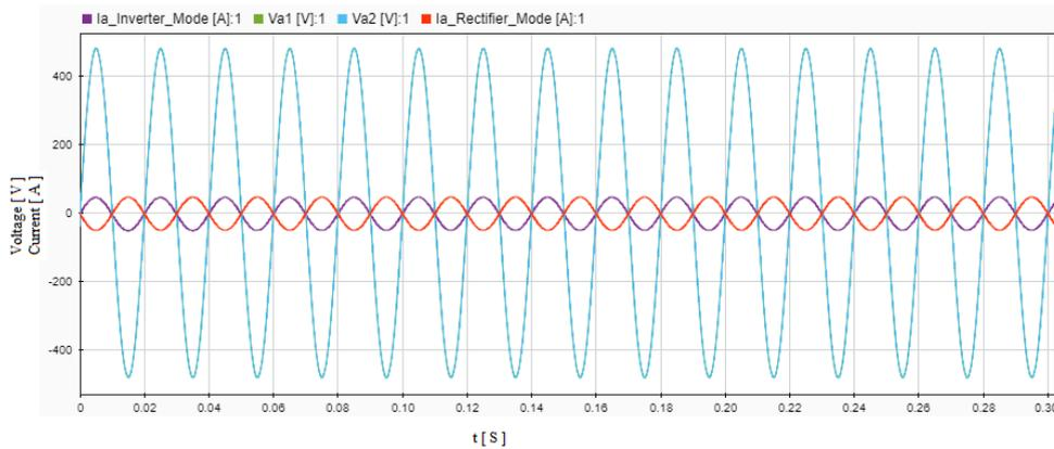
Figure 5.7: AC voltage and current for both rectifier and inverter mode.
