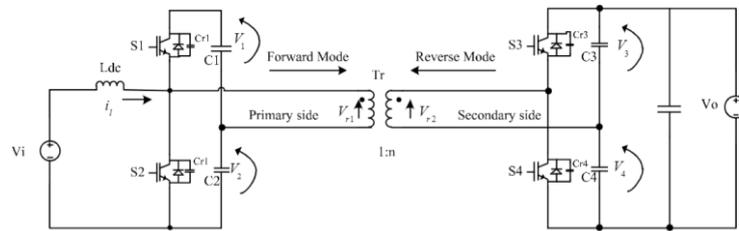
Figure 3.12: Half-bridge bidirectional DC-DC converter [50].
