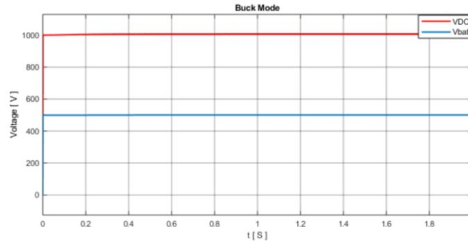
Figure 5.9: Input and Output voltages of the bidirectional DC-DC converter in buck mode.
