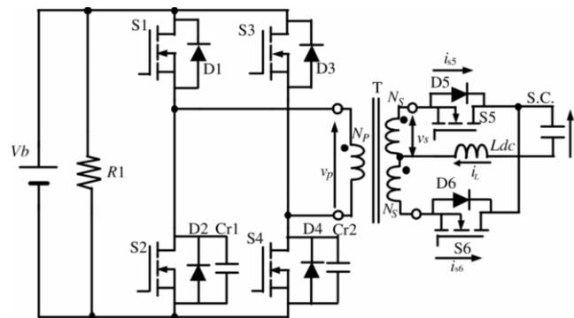
Figure 3.13: Centertapped push-pull bidirectional DC-DC converter [51].
