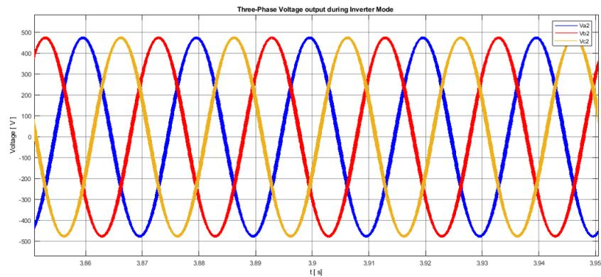
Figure 5.23: Three-phase AC voltage produced by the bidirectional AC-DC converter during discharging.
