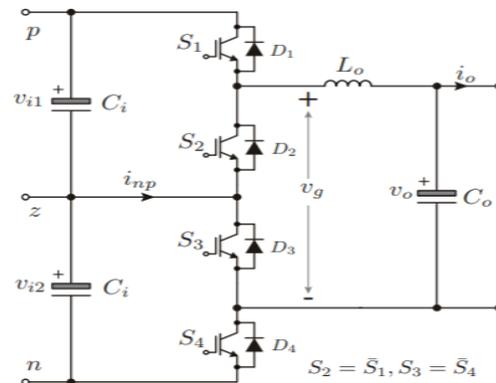
Figure 3.10: Bidirectional three-level DC-DC converter [43].
