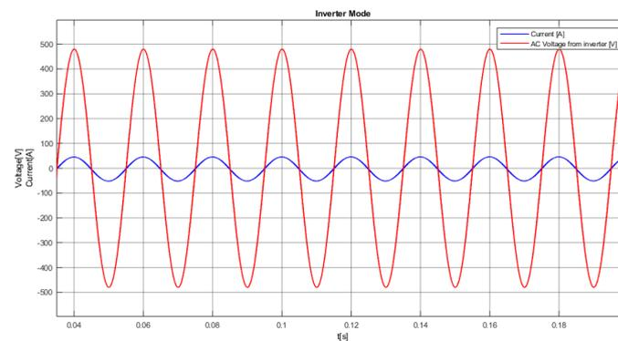
Figure 5.5: AC voltage and current under inverter mode with a  $1^\circ$  phase angle.
