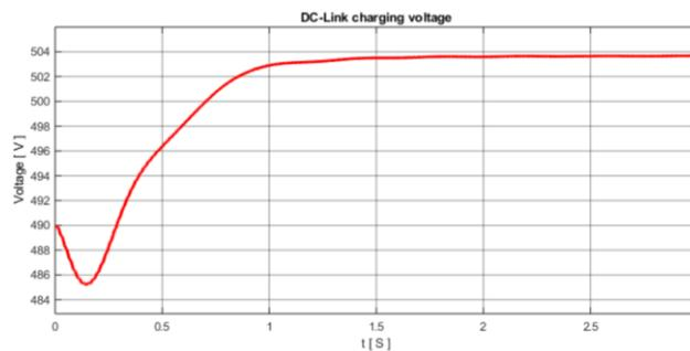
Figure 5.17: Center-taped DC link voltage during rectifier mode.
