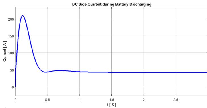
Figure 5.26: DC discharging current at phase angle  $5^\circ$ .
