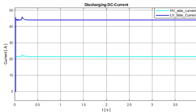
Figure 6.12: Average discharging DC current in the high and low voltage side of the DC-DC converter.
