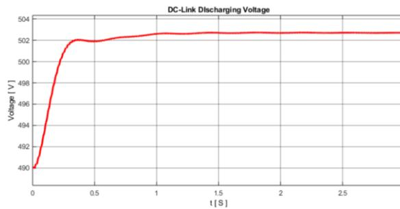
Figure 5.27: Center-taped DC link voltage.
