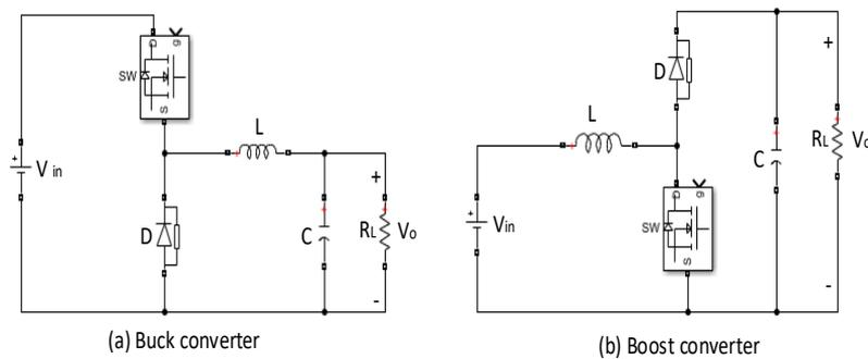
Figure 3.8: Unidirectional buck and boost converters.
