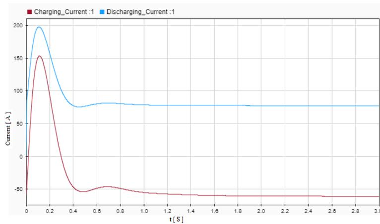
Figure 5.30: Charging and discharging DC current.
