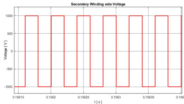
Figure 6.3: High voltage side AC square voltage.
