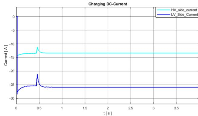
Figure 6.9: Average charging DC current in the high and low voltage side of the DC converter.
