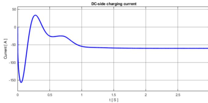
Figure 5.16: Battery DC charging current.
