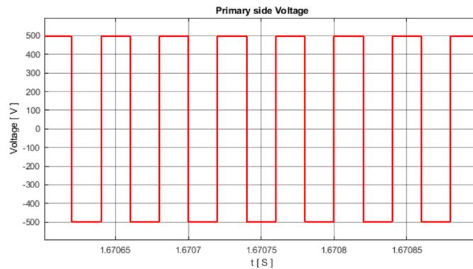
Figure 6.2: Low voltage side AC square voltage.
