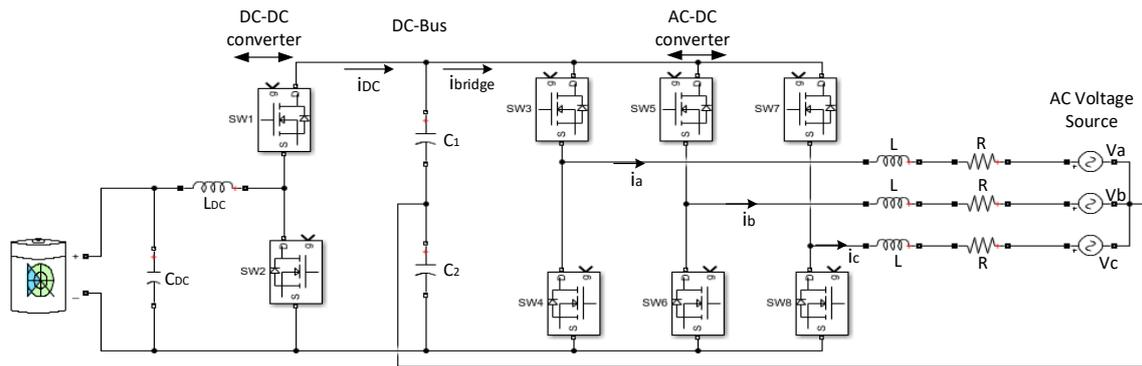
Figure 5.1: A simplified two-stage bidirectional EV charger without galvanic isolation.
