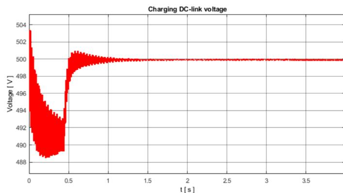
Figure 6.8: DC-link voltage during charging.
