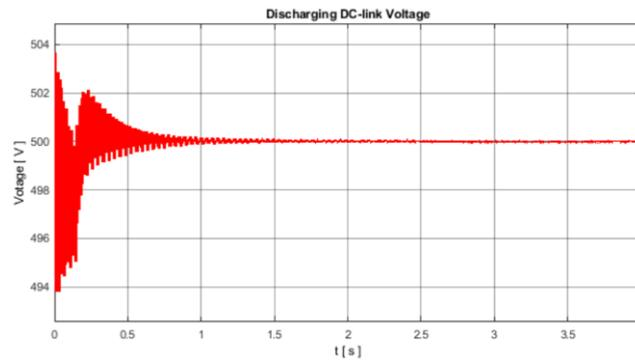
Figure 6.11: DC-link voltage during discharging.
