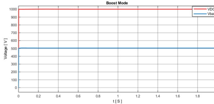
Figure 5.10: Input and Output voltages of the bidirectional DC-DC converter in Boost mode.
