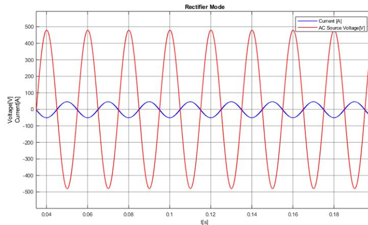
Figure 5.4: AC voltage and current under rectifier mode with a  $1^\circ$  phase angle.
