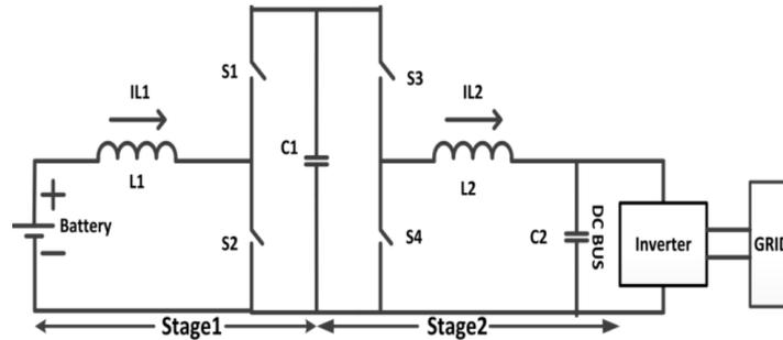
Figure 3.7: Cascade bidirectional DC-DC converter topology[40].
