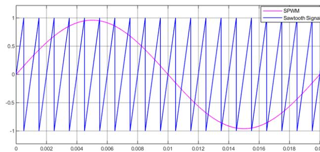
Figure 5.11: Sinusoidal pulse width modulation.
