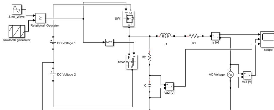
Figure 5.2: Half-bridge single-phase bidirectional AC-DC converter.
