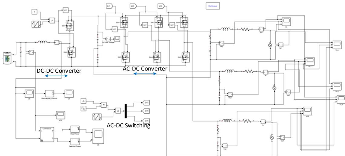
Figure 5.31: Simulation model proposed for EV charger without galvanic isolation.
