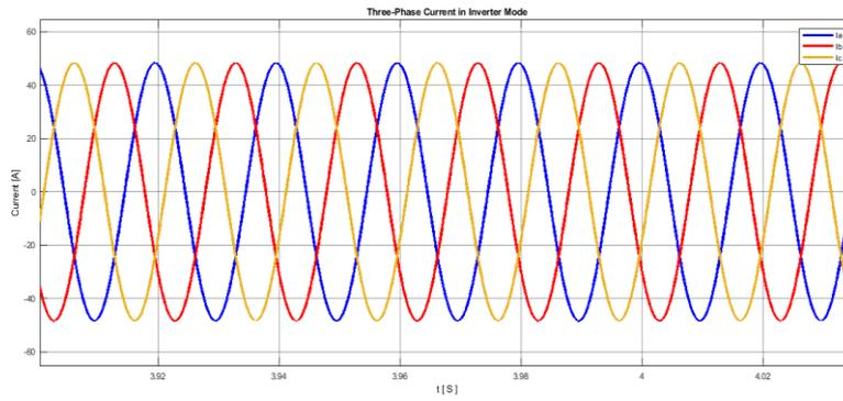
Figure 5.24: Three-phase AC current in discharging mode.
