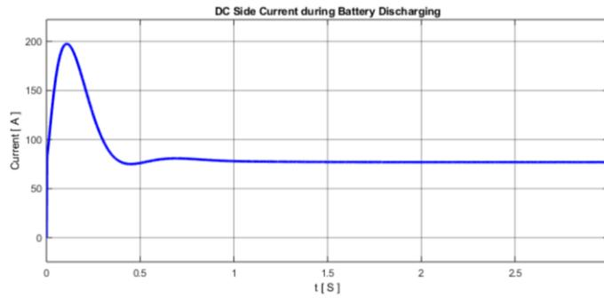
Figure 5.25: DC discharging current at phase angle  $10^\circ$ .
