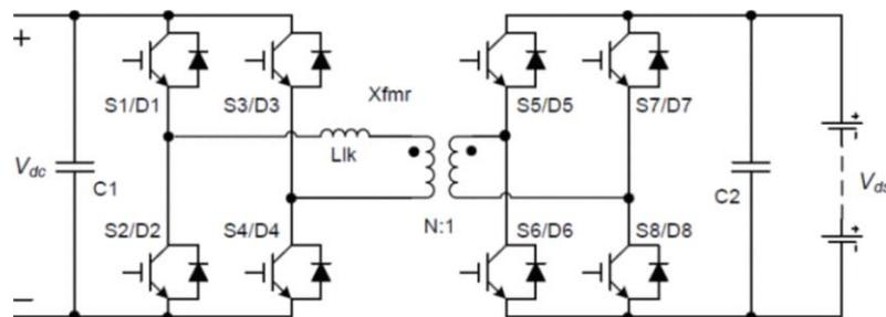
Figure 3.11: Bidirectional full-bridge DC-DC converter based on two voltage-fed [45].
