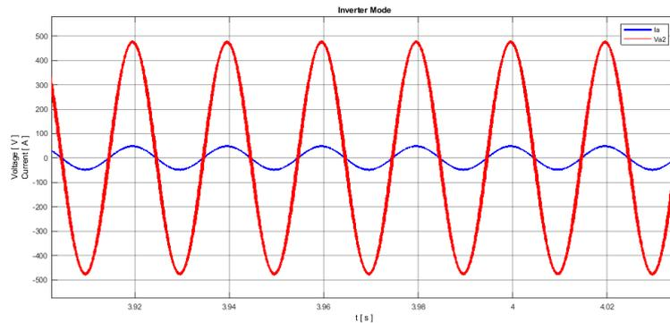
Figure 5.20: AC voltage and current converted by the bidirectional AC-DC converter during discharging.
