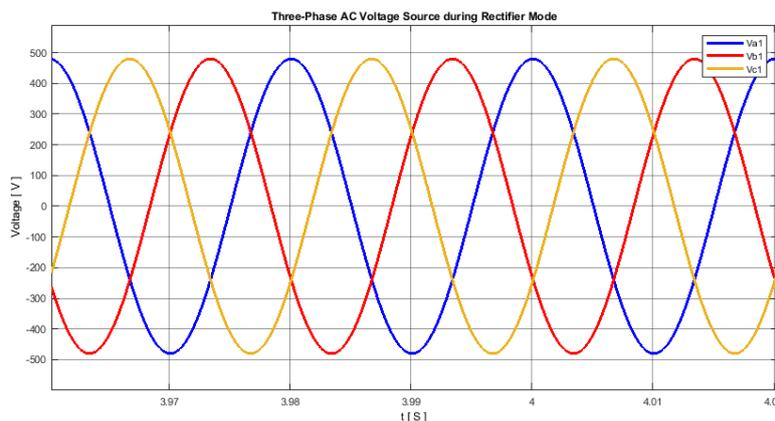
Figure 5.14: Three-phase grid voltages during charging.
