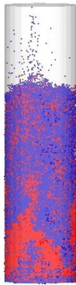
Figure 6.18: Result, Pilot-Scale Gasifier: at a gas velocity of 0.101 m/s.
