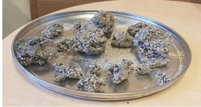
Figure 2.6: Agglomerates from fluidized bed biomass gasification.
