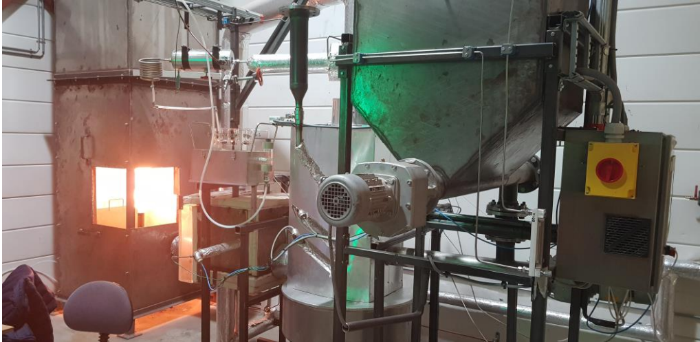
Figure 4.5: Experiment, BFB-gasifier: set up viewed from the right side.
