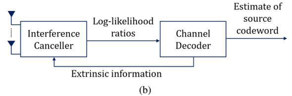
Fig. 4. Block diagrams of: (a) the proposed system; and (b) the conventional one.
