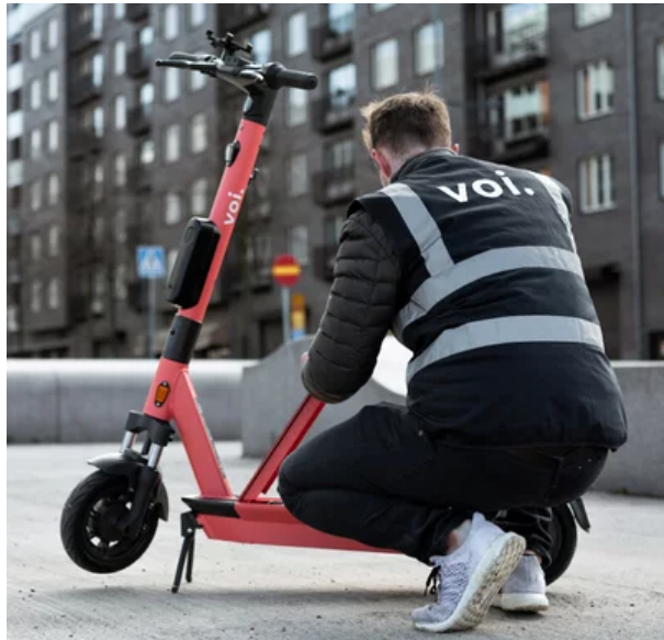
Figure 2.2: VOI scooters. The "black box" in the front is where the hardware is placed. (source:voiscooters.com)
