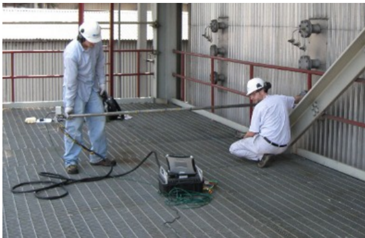
Figure A.8: Full system for measuring flow velocity. Manufactured by Airflow Sciences Equipment, LLC. Photo taken from 3DDASTM Data Acquisition system and Accessories Price List – 2020
