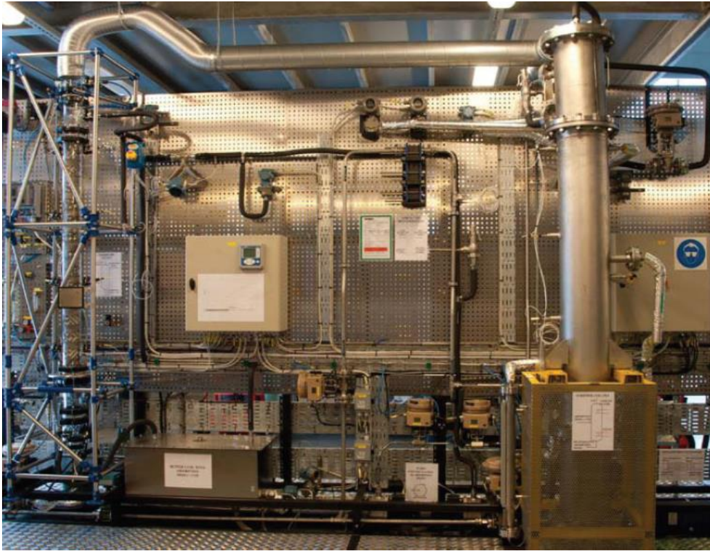
Fig. 1. Amine based post combustion CO 2 capture pilot plat at University of Southeast Norway [1]
