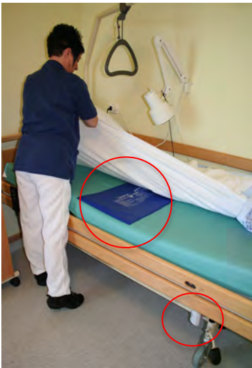
Picture 3-2 Sensor technology for digital monitoring included bed-sensor and beam-sensor mounted on bedframe
