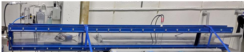
Figure 3.3: Channel setup image viewing the pneumatic valve connected to the release pipe and spark electrodes for ignition
