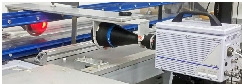
Figure 2.10: The configuration of Shadowgraph system used in the experiments
