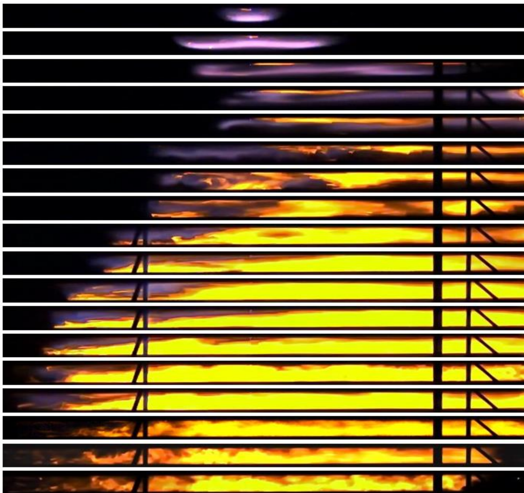
Figure 3.9: Flame propagation during 72 \text{ ms} and 7 \text{ ms} after the ignition of released hydrogen in the channel at a flow rate of 40 \text{ Ndm}^3/\text{min} and release duration of 80 \text{ s} .
