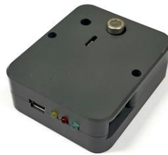
Figure 2.6: Concentration sensors XEN-5320 from Xensor Integration. WIFI read out.
