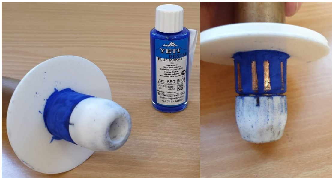
Figure 5-6: Male contact with blue marker
