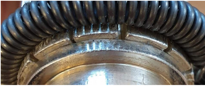
Figure 5-5: Illustration of equally distributed fingers.
