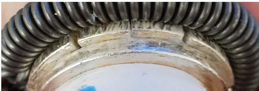
Figure 5-4: Illustration of non-equally distributed fingers.
