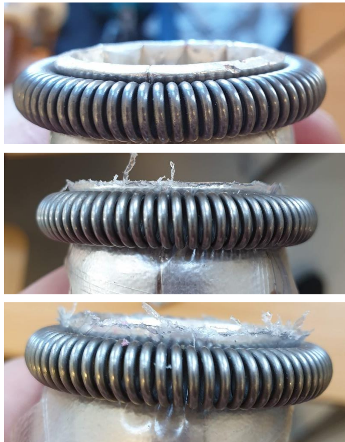
Figure 5-10: Measuring the tulip spring with plastic between spring and fingers.
