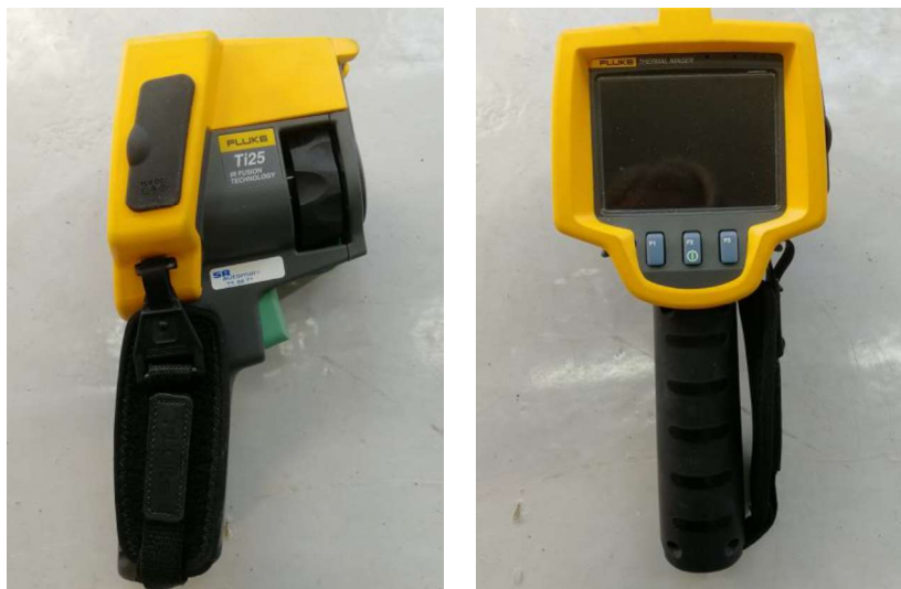
Figure 5.1: The thermal imager from Fluke
