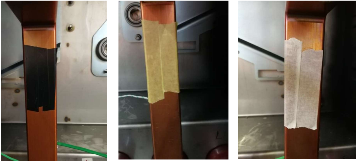
Figure 5.4: Finding the emissivity using three different type of tape
