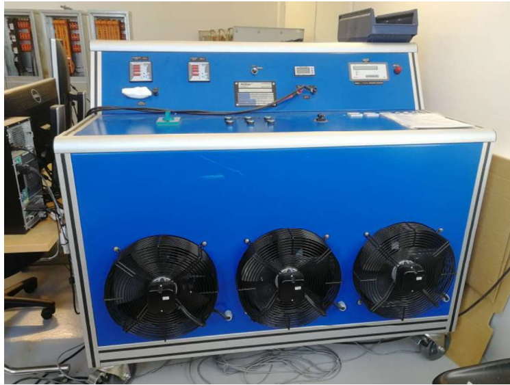
Figure 3.5: Hilkar current injector tester
