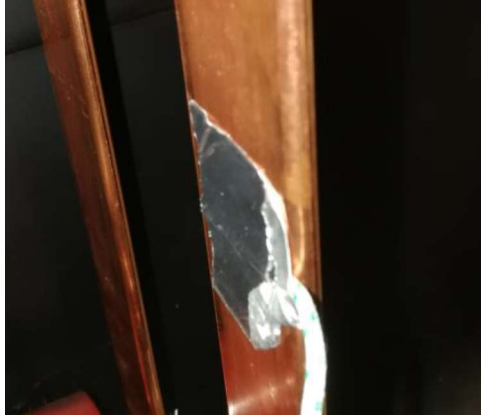
Figure 5.2: Thermocouple elements fastened to the backside of the current path
