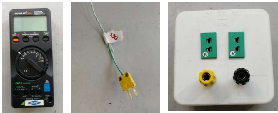
Figure 6.1: METRA HIT multimeter, thermocouple element and a measuring box
