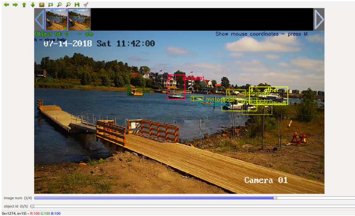
Figure 20 Example of object labeling using YOLO-Mark tool (AlexeyAB, 2019b)
