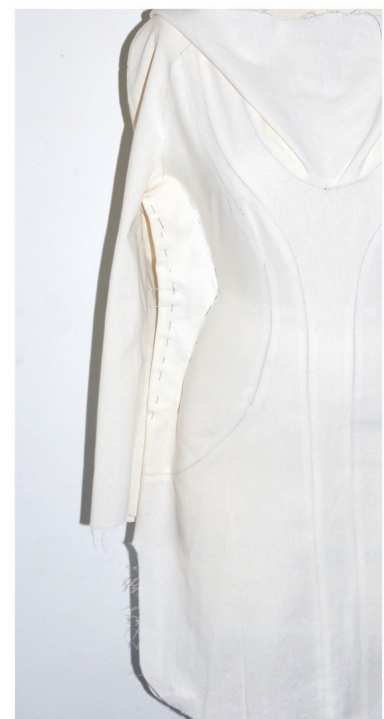
Figure A-10. Toile size small with width reduction by the side seam.
