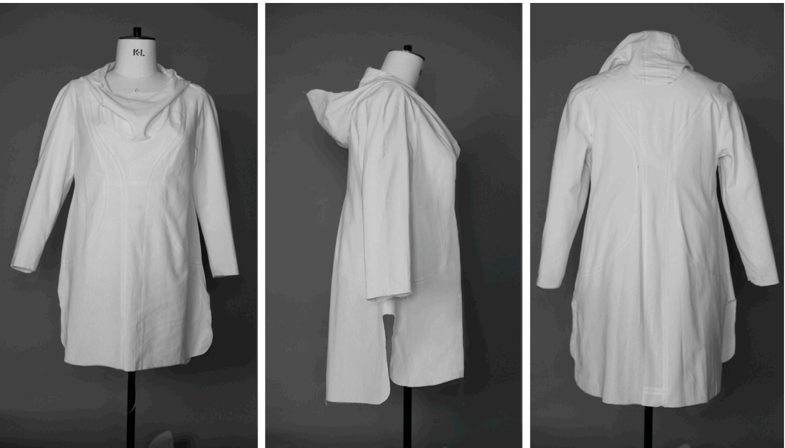
Figure 43. Toile size large sewn with the changes made to the pattern pieces during the fitting.
