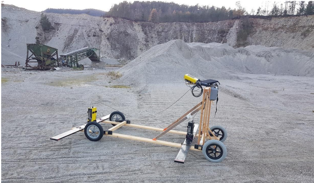
Figure 3-6 - The SmartCart for the 50 MHz antennas with 1.8m spacing. The gravel pit in which the survey took place is in the background.
