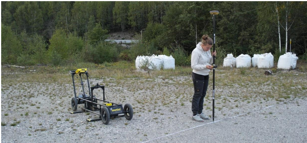
Figure 3-5 - Ingrid Gromstad assisting with the Topcon Hiper-SR GNSS system. To the left is the SmartCart for the 100 MHz antennas with transmitter, receiver and DVL connected.
