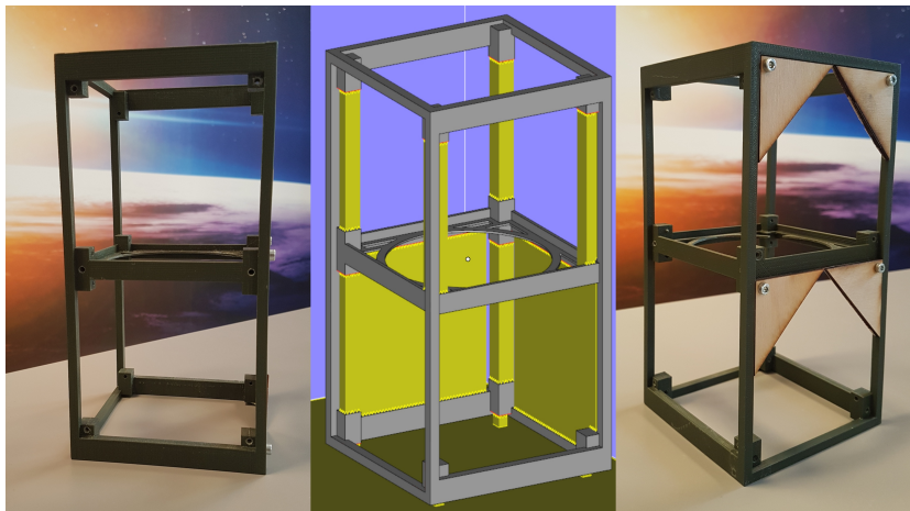
Figure 4.10: The structure of M2 in the orientation it would have been printed.
