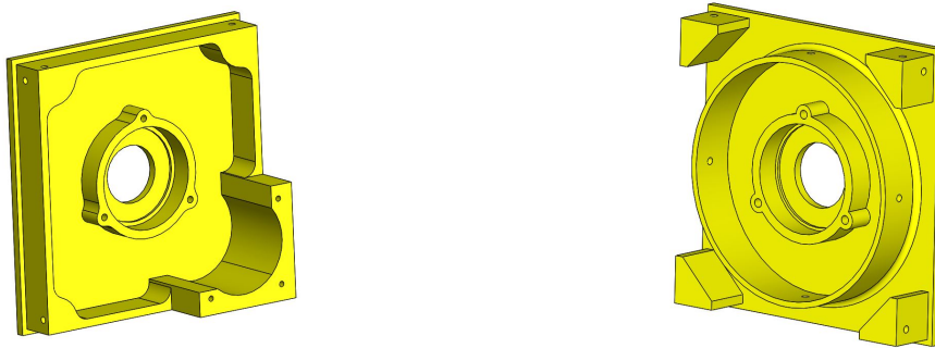
Figure 2: The lids are a part of the primary structure, but also functioning as mounting for Twist Capsule, bearings and the motor.
