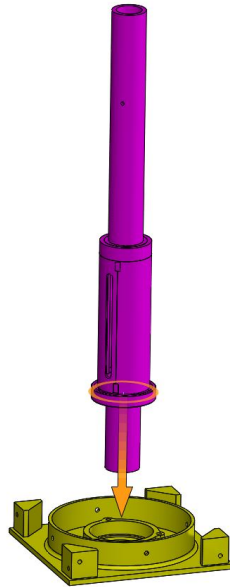
Figure 5: Place the shaft assembly into the Right Lid (item No.1) with the bearing facing the lid.
