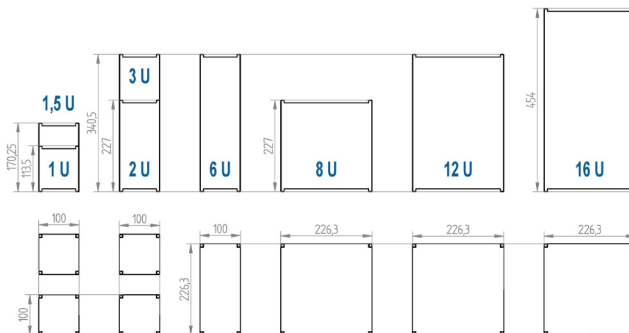
Figure 2.1: The different sizes of CubeSats. Source: ECM-space
