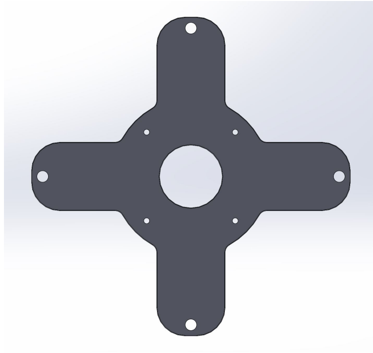
Figure 82: Fixture for electrical motor, P-C3-3.0.4
