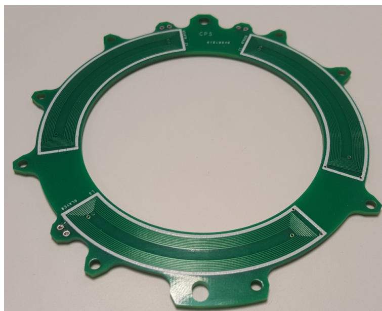
Figure 61: Finished Stator PCB
