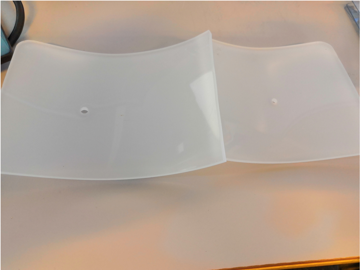
Figure 6.5: Opal white plexiglas first bending test
