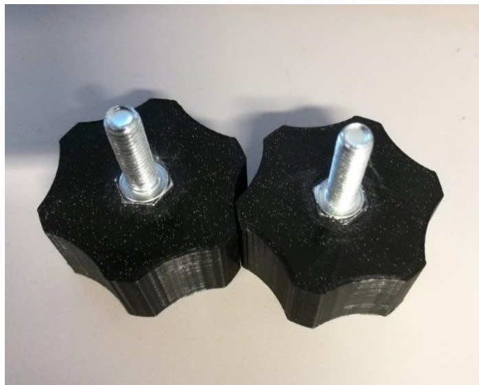
Figure 5.13: Fastener for camera box frames
