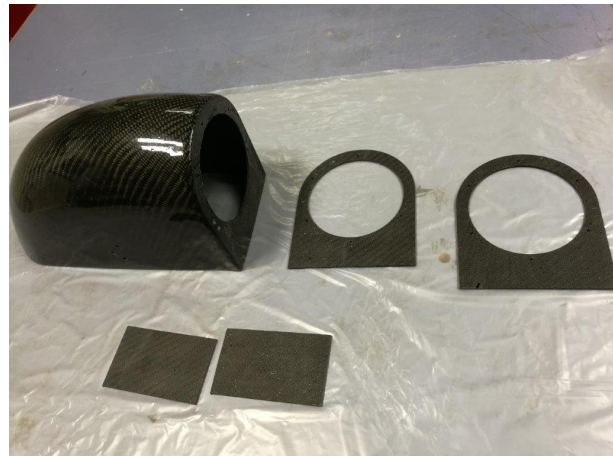
(b) Repair and support pieces ready for adhesive to fix the rear box
