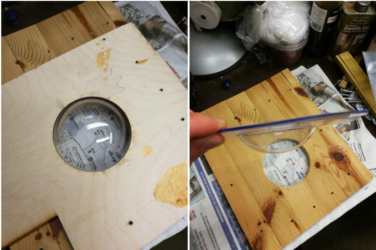
Figure 5.7: First try of blow moulding plastic dome testing if it was possible to blow mould ourselves. Did not achieve sufficient pressure, as mould was not air tight. Did not achieve sufficient size
