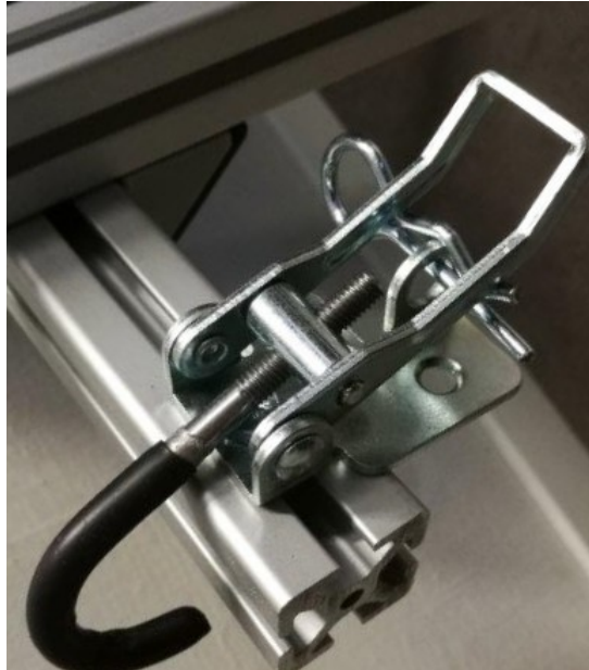
Figure 5.12: Eccentric lock mounted on the roof mounting system
