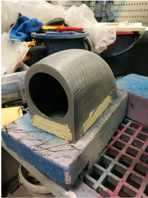
(a) First 3d printed mould with spackle to straighten the warping
