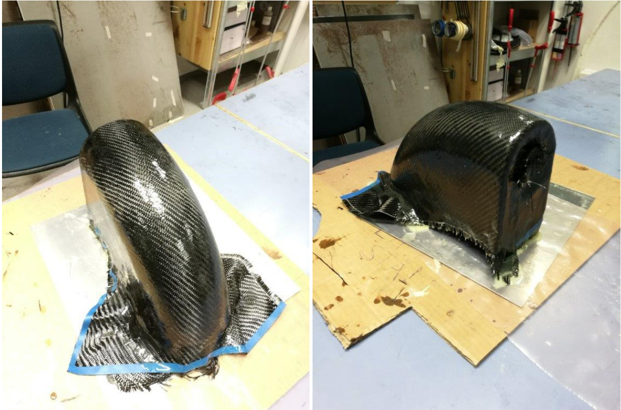
Figure 5.6: Successful casting of the top shell of the rear camera box
