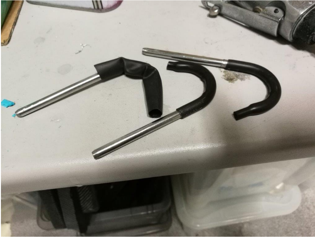
Figure 5.11: Hooks for mounting between roof rack and our mounting system
