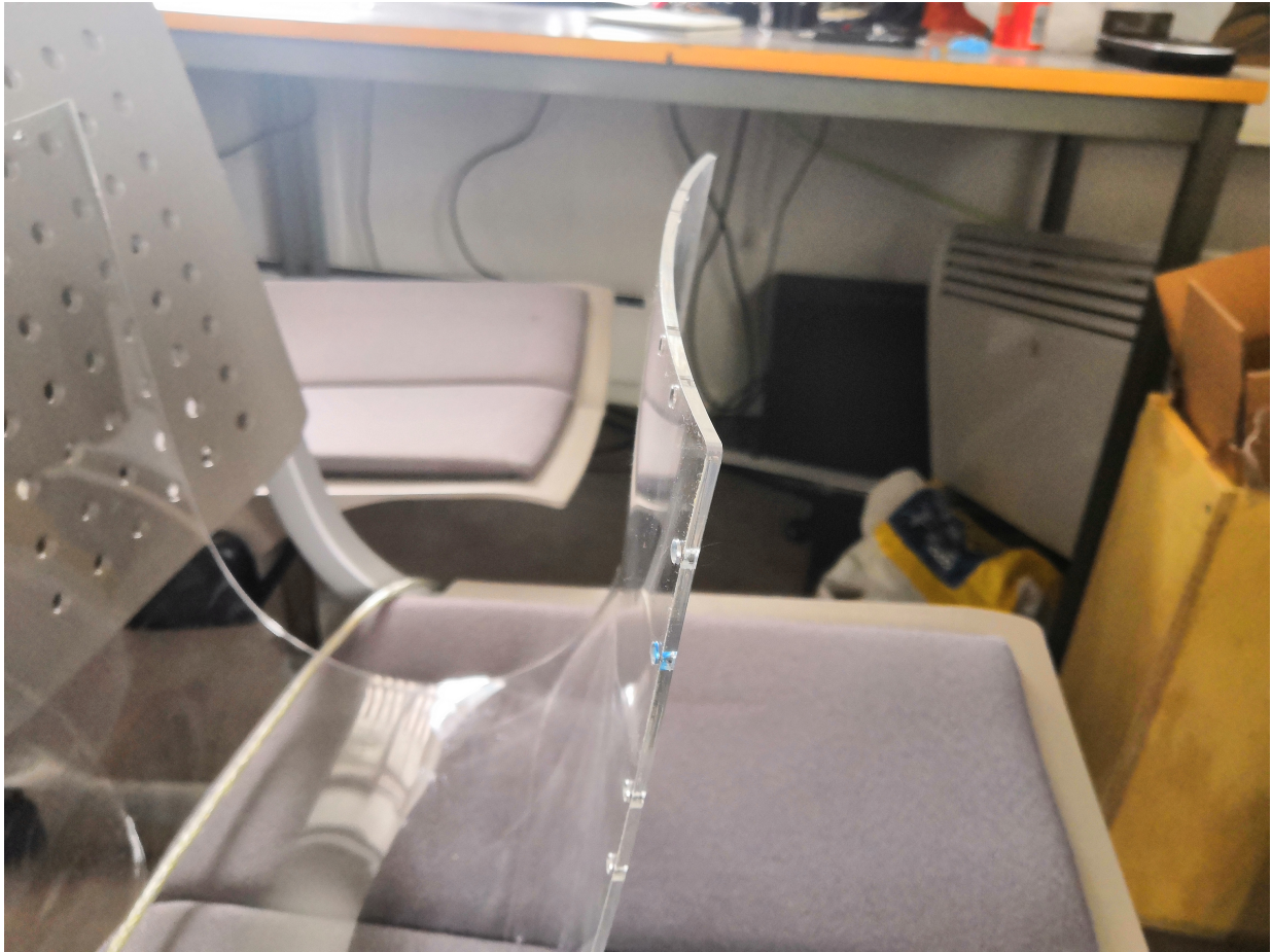
Figure 6.8: Second plexiglas bending warping
