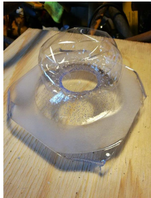
(b) Misshapen dome due to temperature and pressure. Air bubbles has started to form in the material
