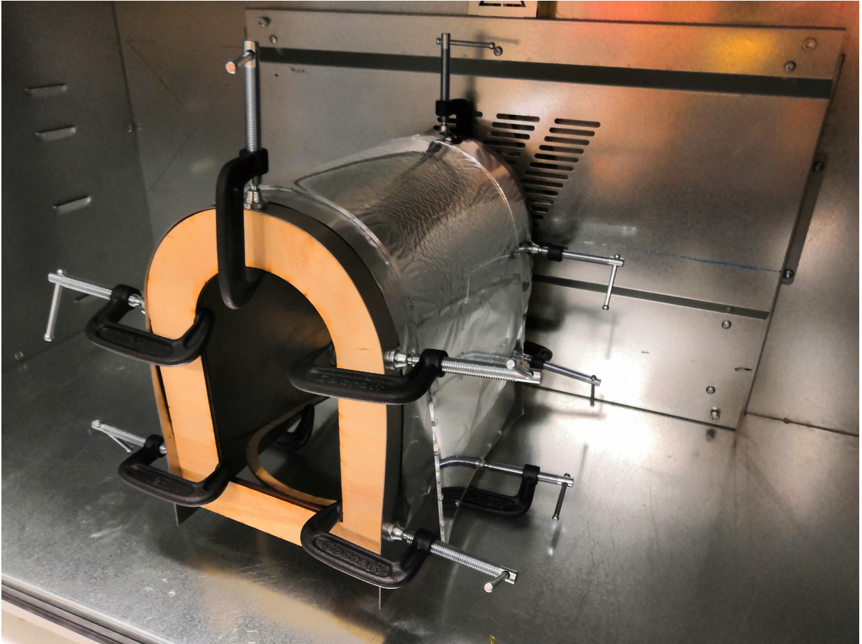
Figure 5.2: Plexiglas mold in oven, warping at the edges of the plexiglas
