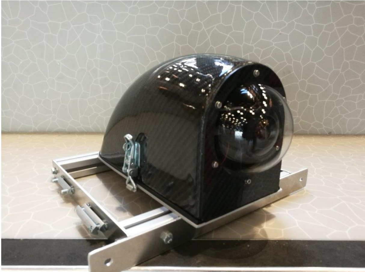
Figure F.2: Produced rear camera box for the Argos system
