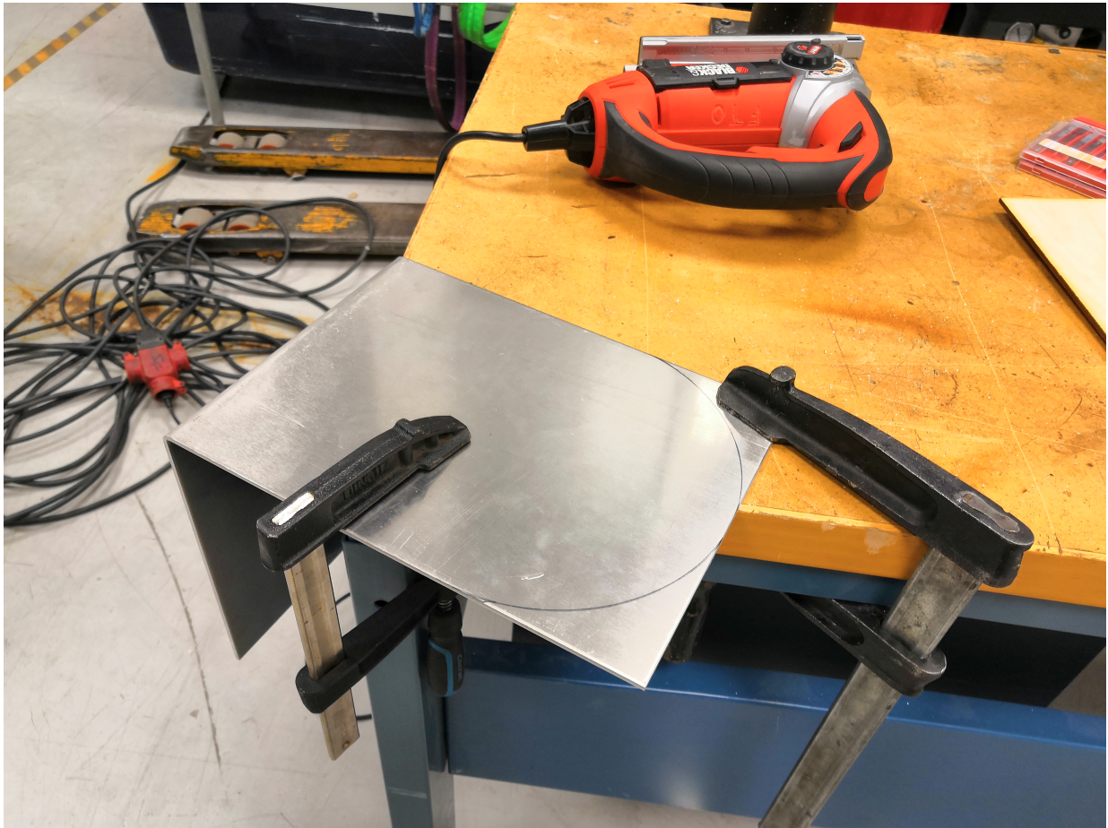
Figure 5.3: Front camera box lid jigsaw cutting
