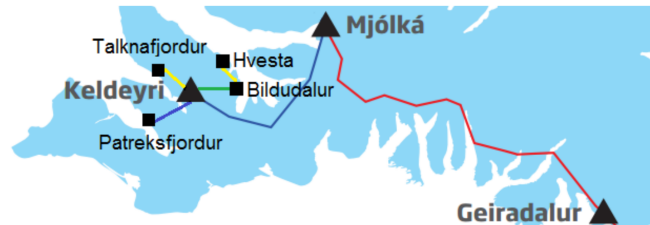
Figure 1. Overview of the transmission system with voltage levels: 132 kV 66 kV 33 kV 11 kV
