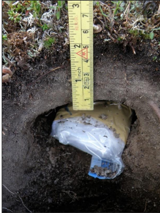
Figure 7: Placement of a datalogger in the soil.
