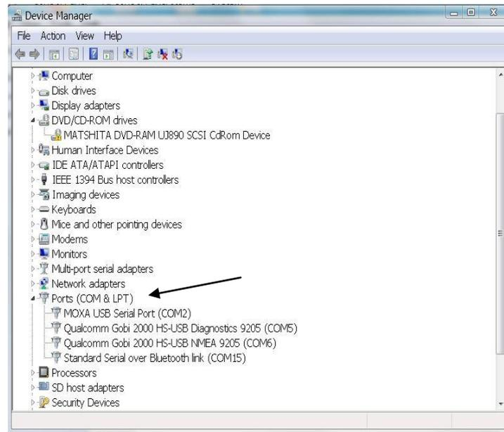
Figure a: Demonstration of ports
