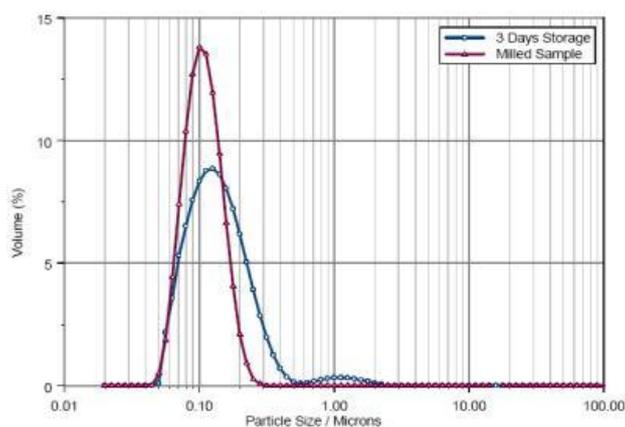
Figure 2.7: Particle size distribution [28]
