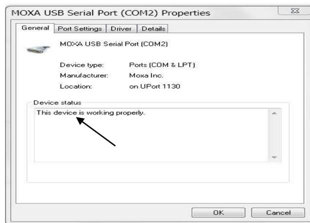
Figure b: Verification of working
