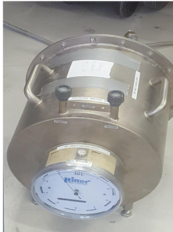
Figure 3-2 Drum-type flowmeter used to calibrate the rotameter used in the experiments
