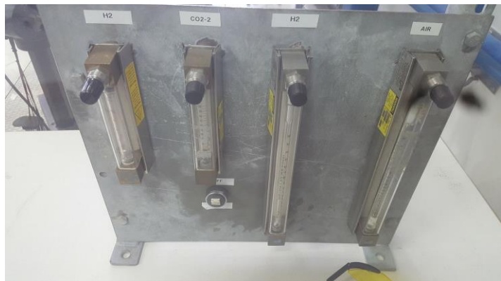
Figure 3-1 Control board. Controls the flow of hydrogen, and whether the flow goes into the combustion chamber, or the bypass into the ventilation
