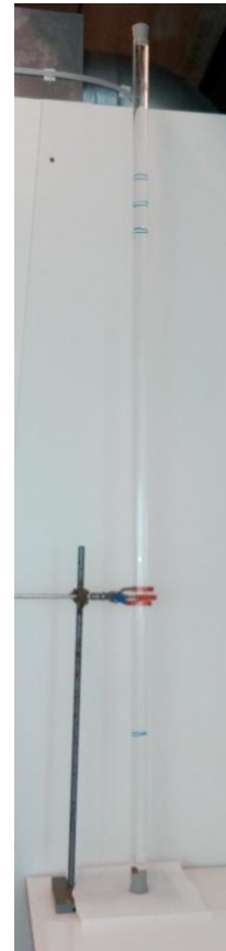
Figure B-17: Plexiglass settling column filled with cooled (5 °C) nonfiltered sea water
