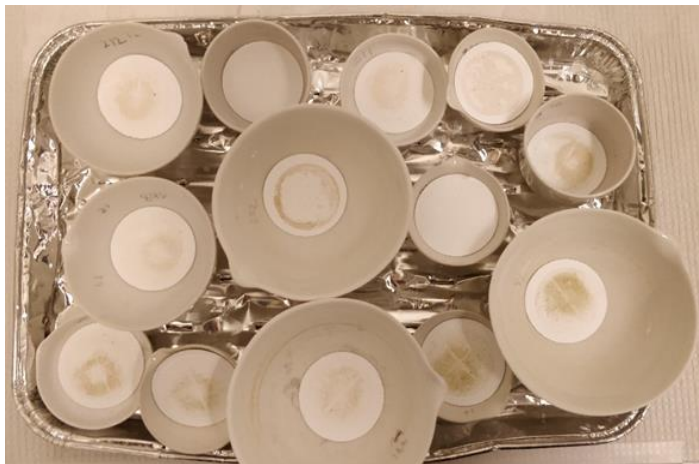
Figure B-16: Filter papers with retain particles (after BOD) after putting into muffle furnace
