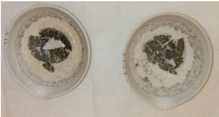
Figure B-3: Fish waste sample after putting into muffle furnace (VS)
