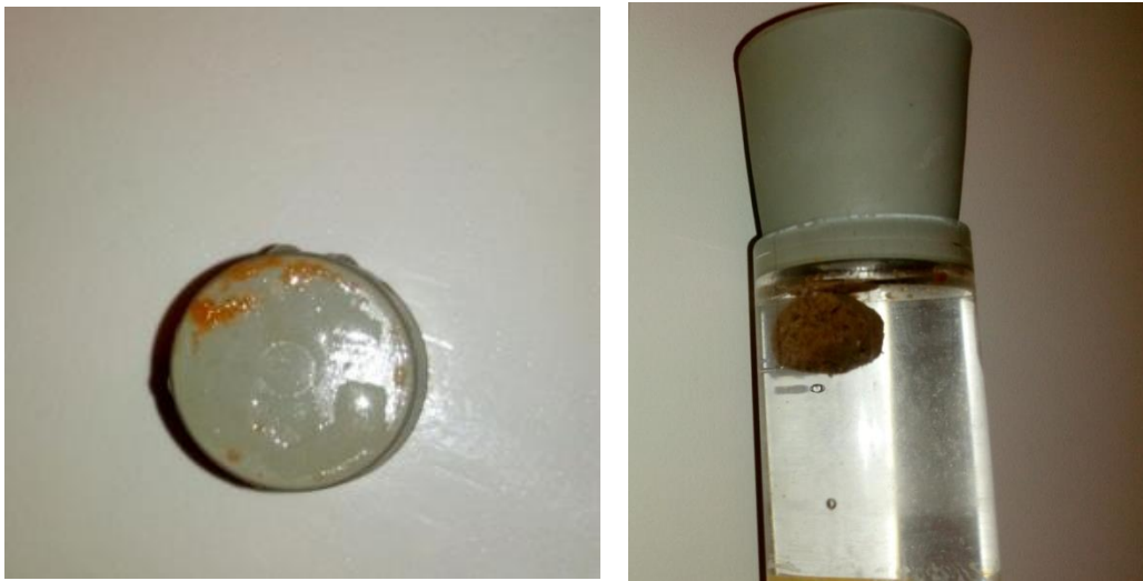
Figure 4-27: Fat bubbles floating on the top of tube for P 1000 and P 500
