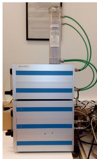
Figure B-14: Sample pump, sample dryer and data collection system for Micro-Oxymax
