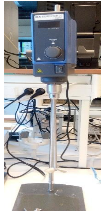
Figure B-2: Electrical agitator
