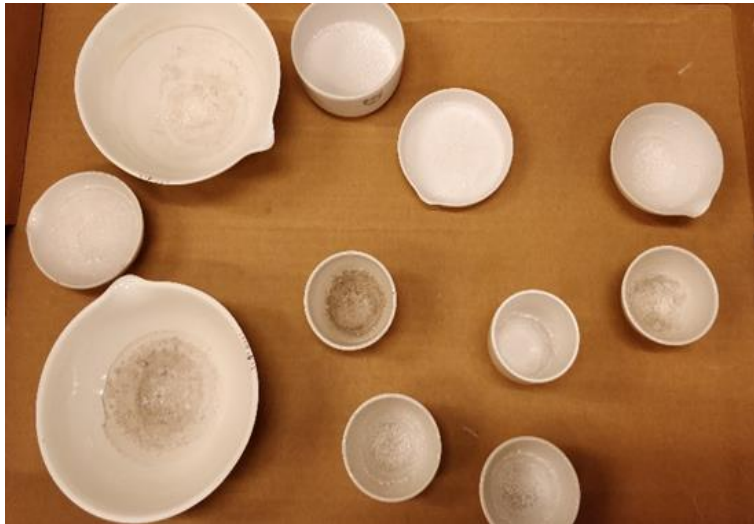
Figure B-15: Samples (after BOD) after putting into muffle furnace
