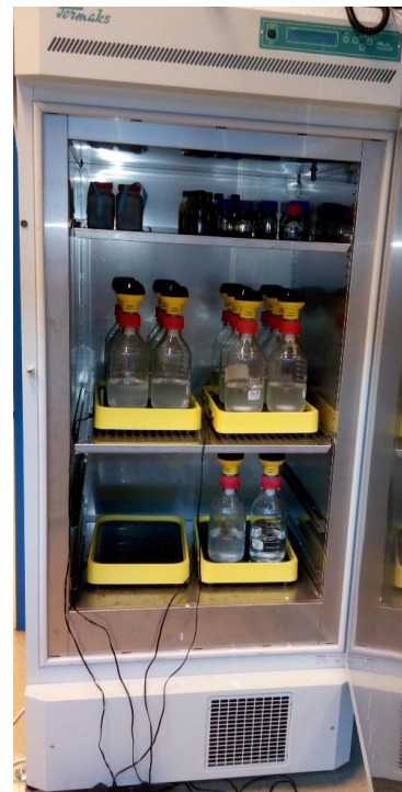
Figure B-10: Bottles on stirring platforms inside an incubation cabinet
