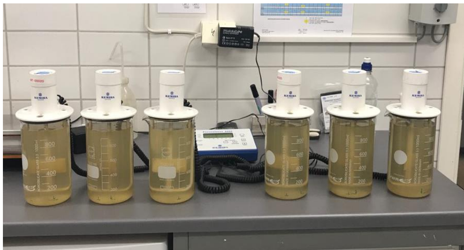
Figure 3-3. Jar test setup which include 6 beakers which are filled with 1 L of wastewater according to the aforementioned proportions
