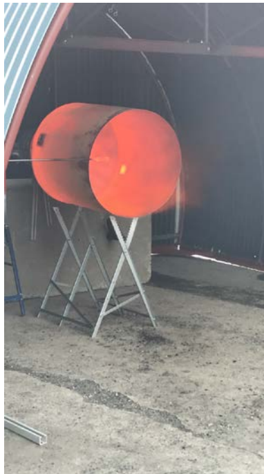
Figure 5.5: Test run with combustion chamber. Indication of heat release from the burner.
