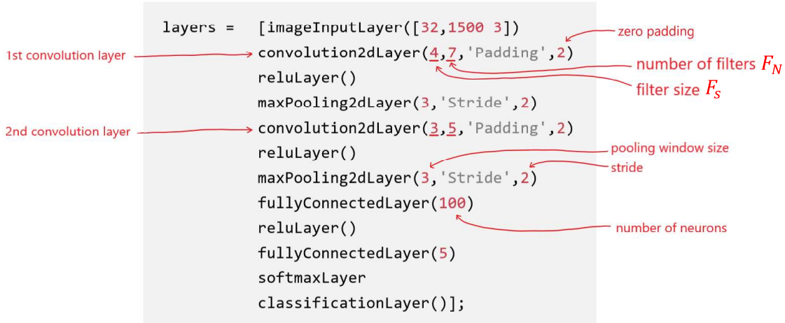
Figure 5.2: Example of how the layers of a CNN can be defined in MATLAB.
