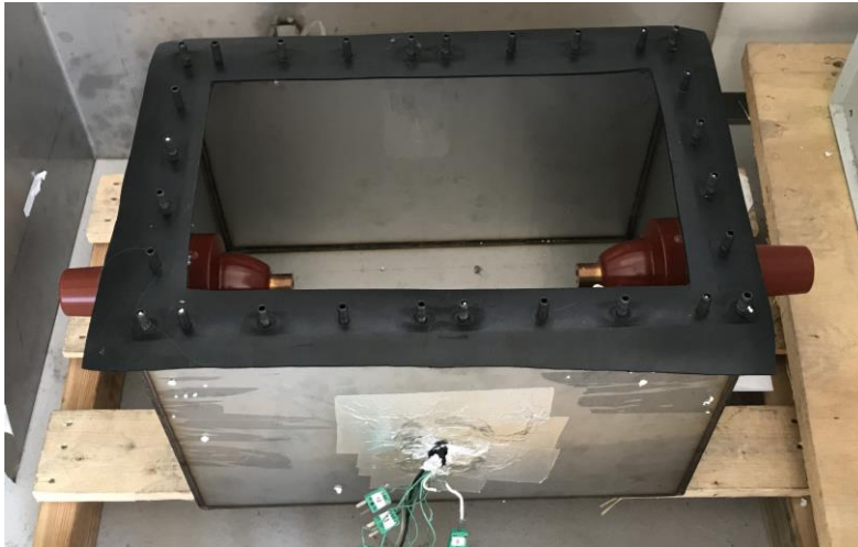
Figure 3.4 – Overview of the small enclosure that fits exactly one switch
