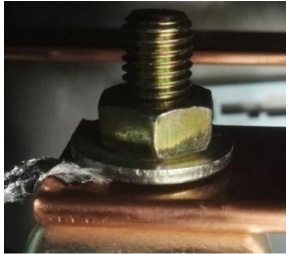
Figure 4.2 – Mounting of thermocouple using the washers beneath the bolt
