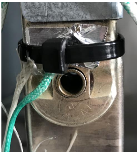
(a) Thermocouple on the rotating contact
