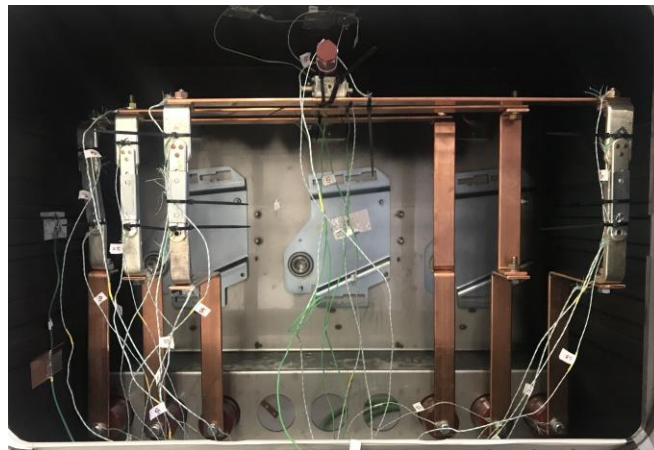
Figure 4.6 – Picture of the finalized test device seen from the front
