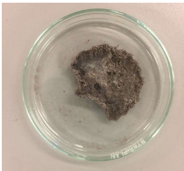
Figure C5: residue left from experiment N8 inside the reactor
