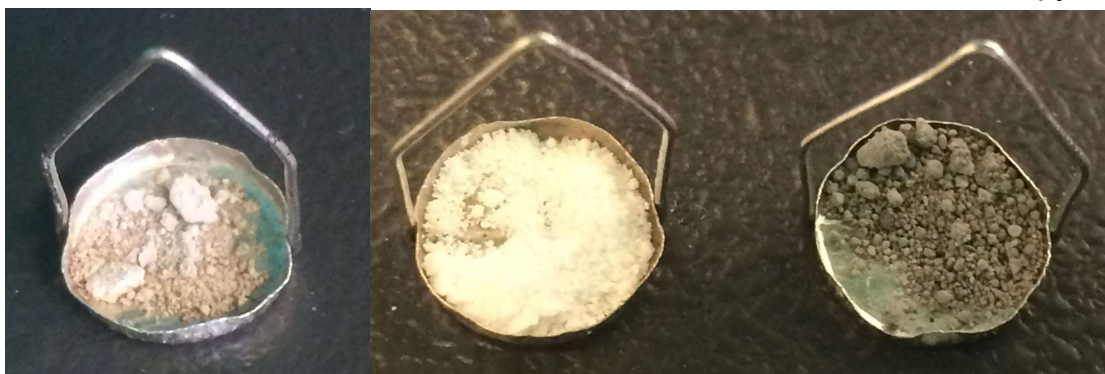
Figure 4.9: From right to left: spent catalyst, catalyst sample subjected to air and catalyst subjected to nitrogen during TGA test
