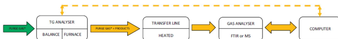
Figure 2.5: A schematic diagram of TGA-FTIR and TGA-MS system [36]
