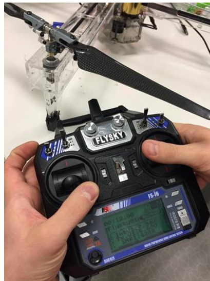
Figure 40: Pitch angle changed on RC
