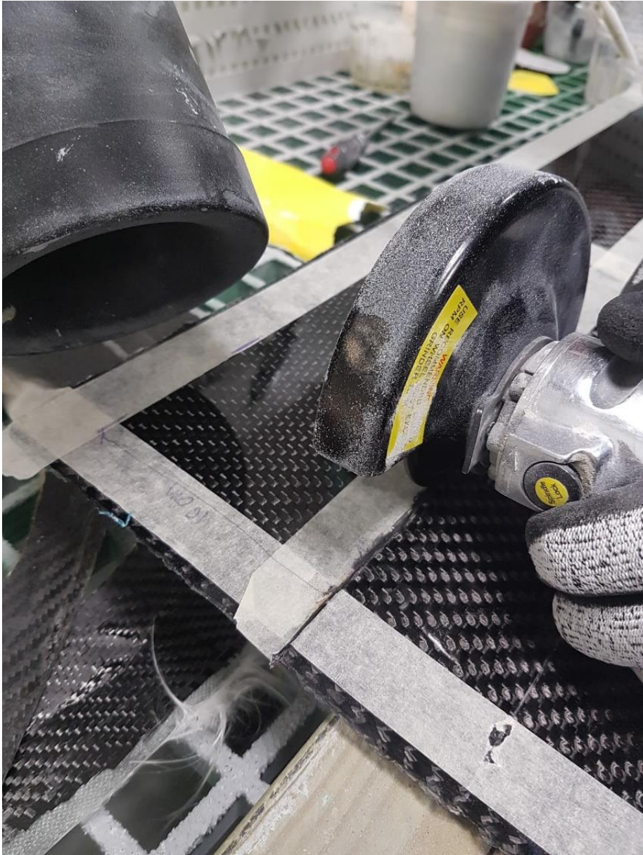
Figure 2.18: Trimming the carbon fiber plates into smaller pieces
