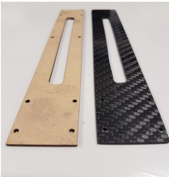
Figure 2.36: MDF and carbon fiber arms
