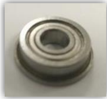
Figure 4.15: The propeller shaft bearing
