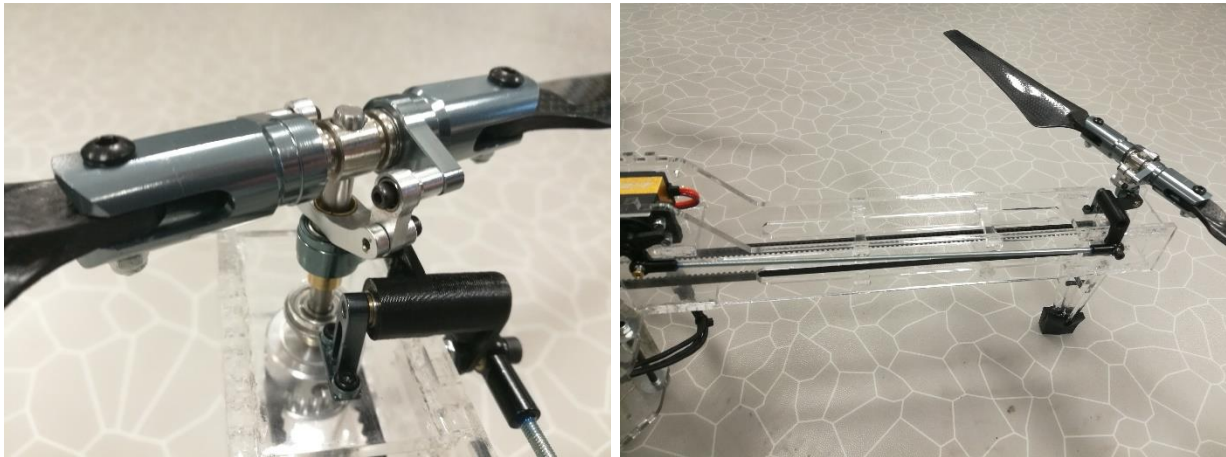
Figure 26: The variable pitch mechanism
