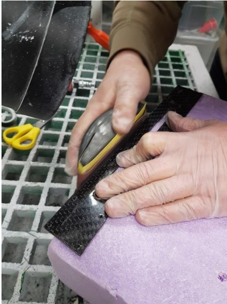
Figure 2.34: Grinding the plates with sandpaper
