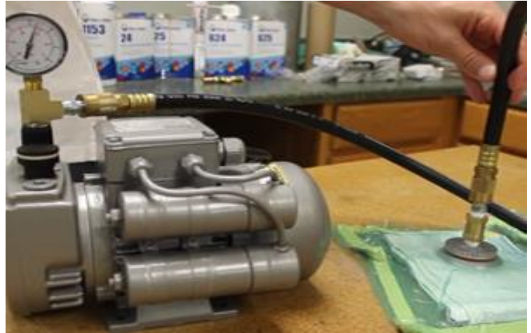
Figure 2.2: Vacuum bagging system
