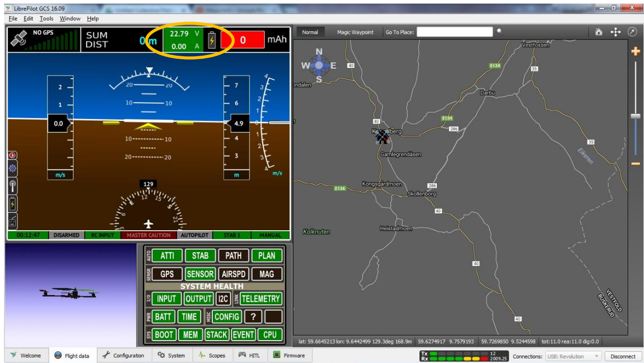
Figure 12.6: Screenshot of the GCS with battery voltage showing in the highlighted circle
