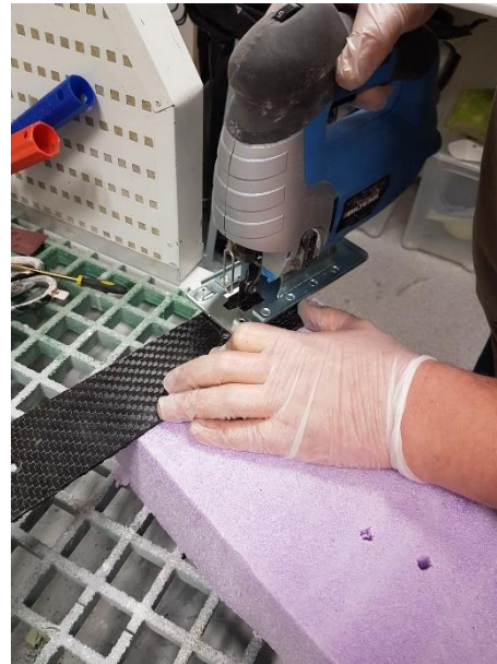
Figure 2.33: Cutting plate with jigsaw
