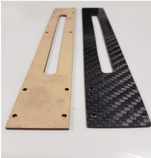
Figure 6.3: MDF and carbon fiber arms
