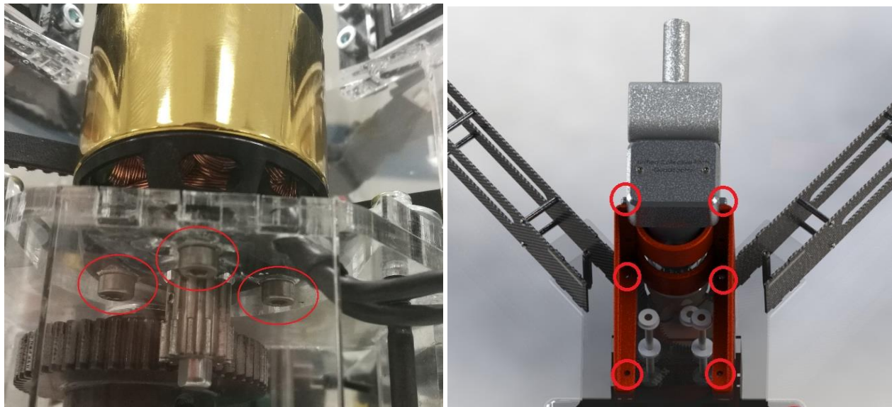
Figure 15: Fastening of the EM and ICE drive units
