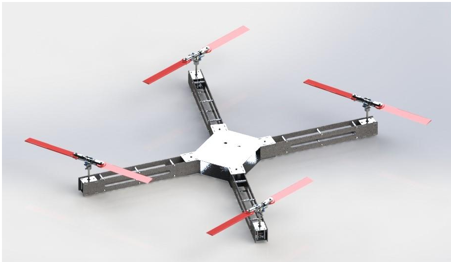
Figure 6.1: SW model of frame in composite
