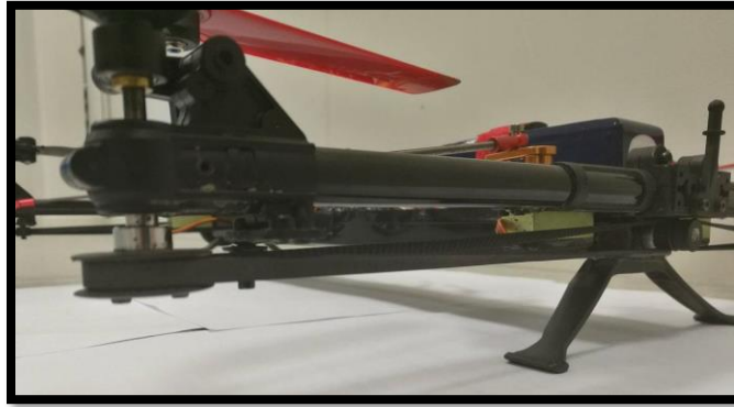
Figure 3.1: Twisted belts of the commercial WL-toys-v383 quadcopter
