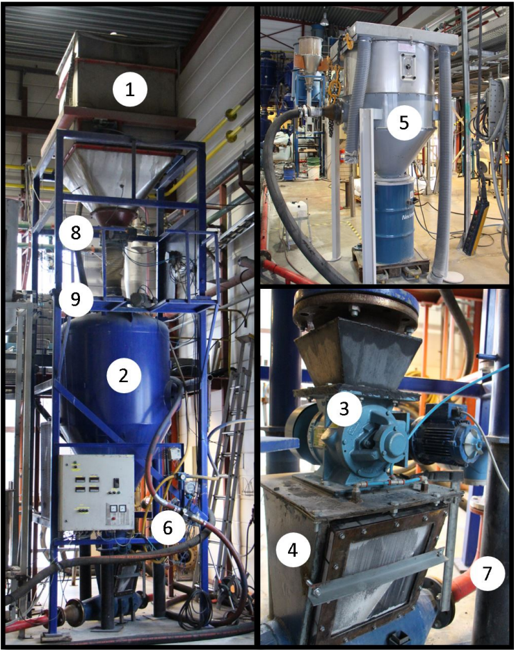
Figure 3.6: Storage and receiving tanks of the conveying rig
