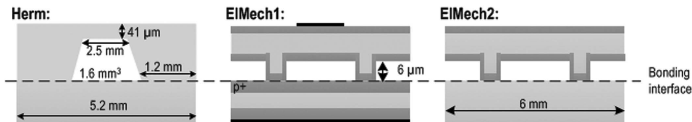
Figure 1. Schematic cross-sections of Herm and ElMech dies. Light gray is silicon, dark gray is p + -doped silicon, black is aluminum.
