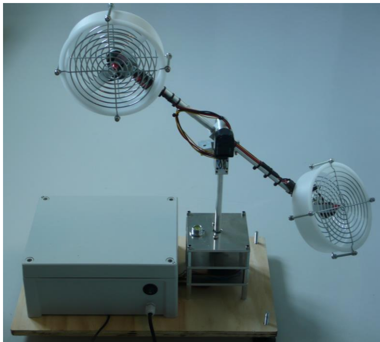
Figure 1-1: Picture of the two degrees of freedom helicopter model built at USN.
