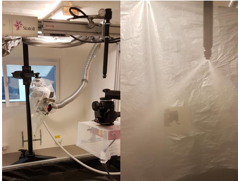
Figure 4-4 Picture of the burner lance, high-speed camera and laser. Picture to the right shows the sprays at initial pressure
