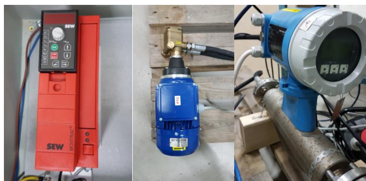
Figure 4-5 Frequency controller, gear pump, and a Coriolis meter for mass flow measurement of water
