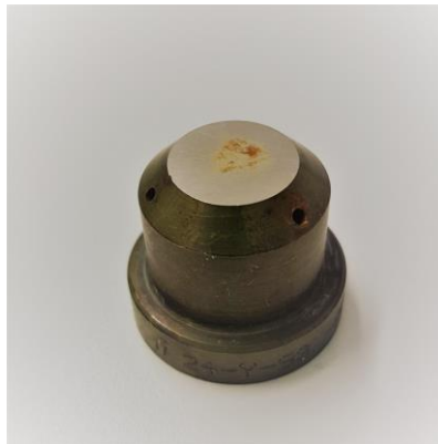
Figure 1-3 Atomizer 24-Y-90°-00-3 from Fluidics Instruments, look to Appendix F Nozzle 24-Y for technical information.
