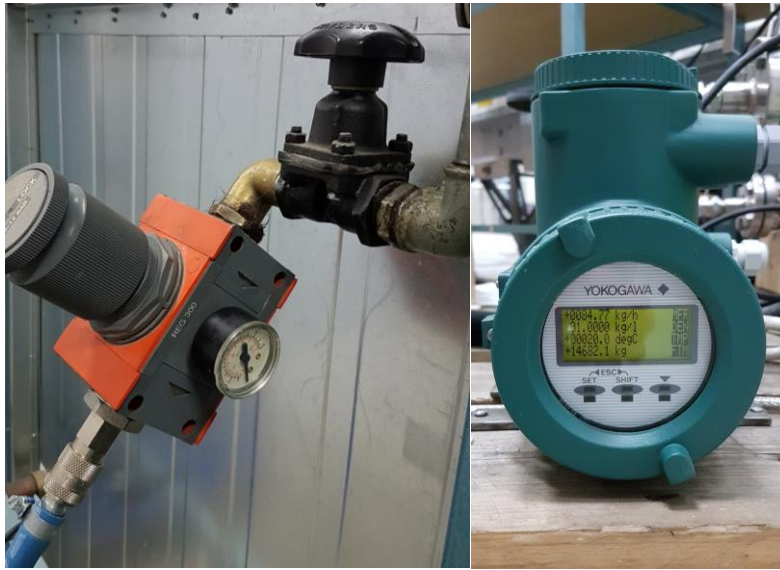
Figure 4-6 Regulator for air supply and Coriolis meter for air mass flow measurement
