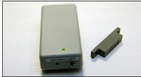
Figure 5-6. A door alarm commonly provided by the local care services which registers if a door is opened and can be turned on and off [6]
