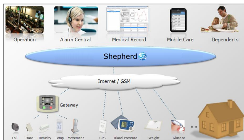
Figure 5-7. Overview of the actors (top), devices (bottom) and communication systems involved the Shepherd data acquisition platform 'Shepherd' by a Norwegian telecommunication vendor Telenor Objects. The figure is translated from [49]
