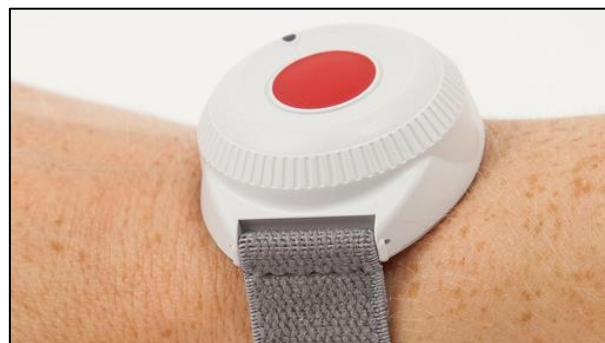
Figure 5-5. A fall sensor of type "Vital Base" that both automatic and manually triggers an alarm. It includes a sensor for movement and one for fall detection [46]
