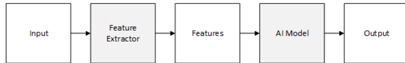
Figure 2-2. Typical flow of activities when creating AI models in use for determining outputs. White boxes indicate parameters and grey boxes indicate algorithms or models for processing and determining parameters
