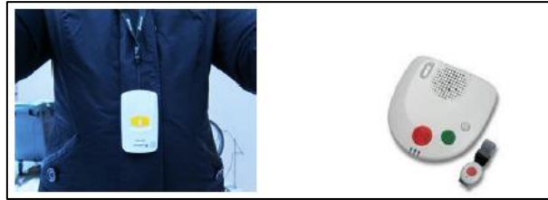
Figure 5-4. To the left, a mobile safety alarm of type 'Safemate', carried around the neck which includes GPS tracking and mobile communication versus a more commonly stationary safety alarm, to the right, that cannot be applied outside the living area [21]
