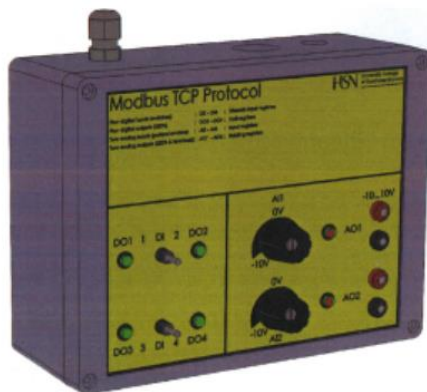
Figure 1: The IoT device with a set of digital and analog inputs and outputs.
