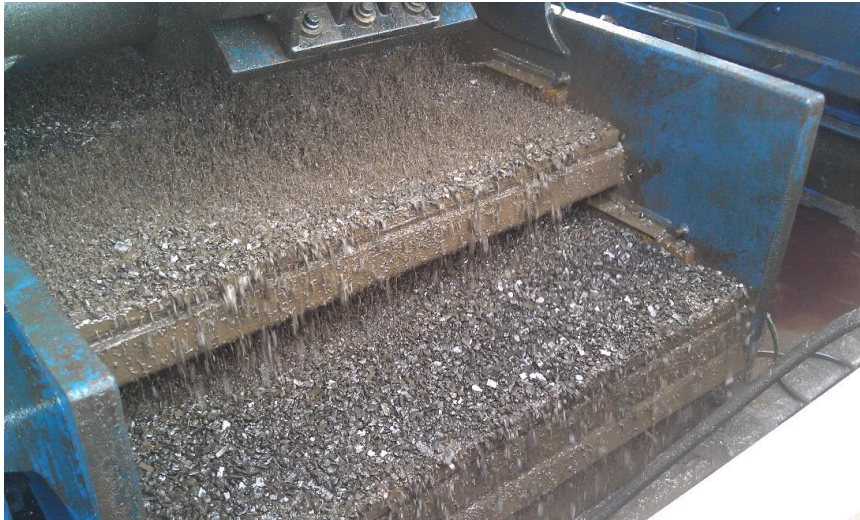
Figure 3-7 Waste from a shale shaker [20]
