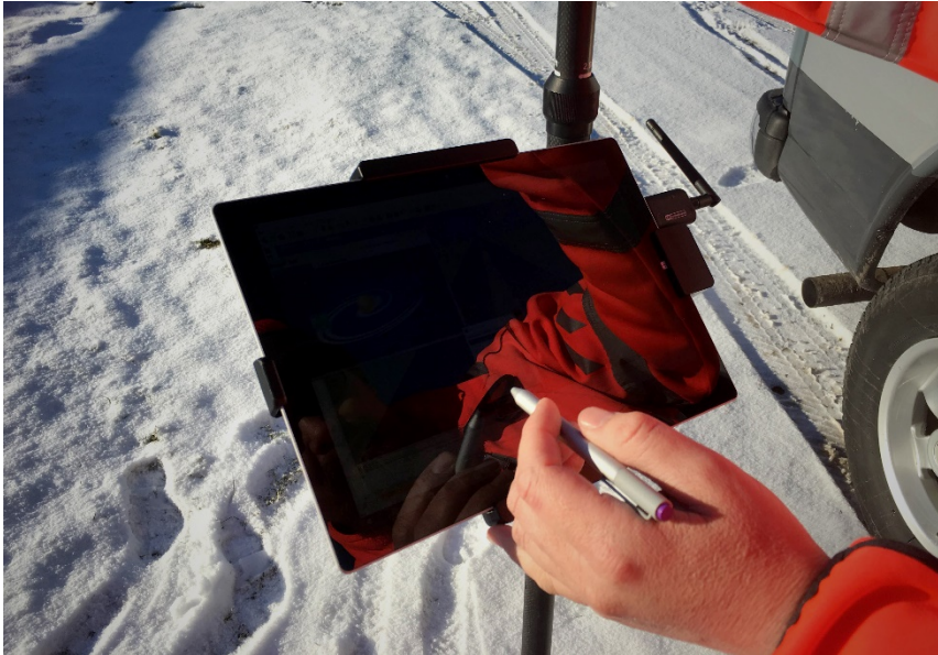
Figure 4-3: Windows surface tablet with registration software
