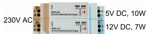
Figure 4.7: Power supply from Carlo Gavazzi in both 10 W/12 V and 7 W/5 V variation. 12 V for Arduino I/O and DAC, 5 V for Raspberry Pi 2 and real time clock.
