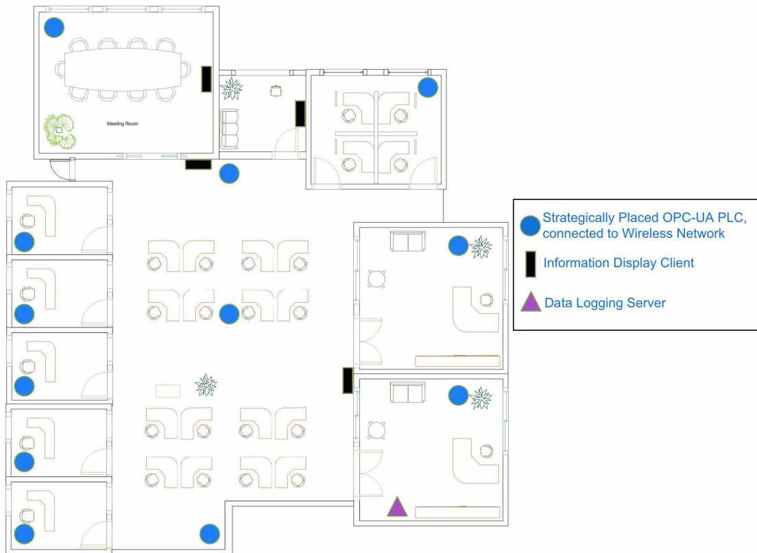
Figure 2.6: Overview of the office floor, showing the twelve PLC units, four information displays and one data logging server.
