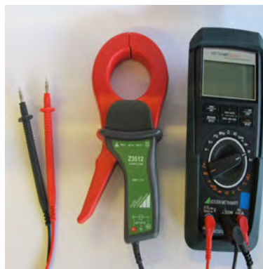
Figure B.5: Probes and coil for measuring the watt
