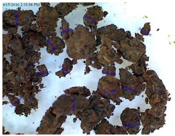
Figure 4-5. The VMS-001 USB microscope picture and the measured diameter of coffee grit 2 with the range from 0.35 – 1.23 mm.
