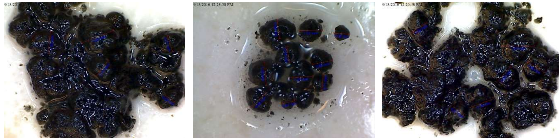
Figure 4-10. The VMS-001 USB microscope picture and the measured diameter of granules sampled from Saugbrugs (new) with the range from 0.58 – 1.73 mm.
