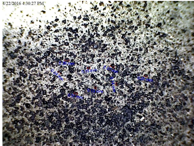
Figure 4-23. The granular size distribution of Saugbrugs (old) exited at 5.2 m h -1 up-flow velocity with range from 0.14 – 0.32 mm.
