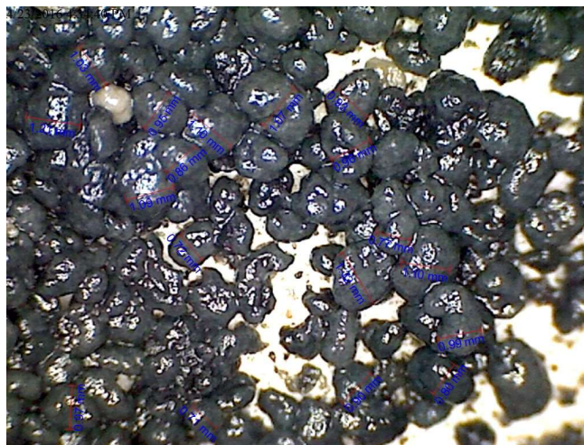
Figure 4-40. The granular size distribution of Saugbrugs (new) exited at 44.7 m h -1 up-flow velocity with range from 0.79 – 1.48 mm.
