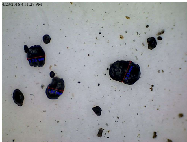
Figure 4-42. The granular size distribution of Saugbrugs (new) exited at 187 m h -1 up-flow velocity with range from 1.17 – 1.71 mm.
