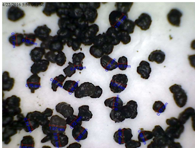
Figure 4-28. The granular size distribution of Saugbrugs (old) exited at 44.7 m h -1 up-flow velocity with range from 0.46 – 1.20 mm.
