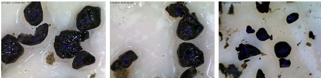
Figure 4-7. The VMS-001 USB microscope picture and the measured diameter of granules sampled from HyVAB reactor with the range from 0.52 – 2.25 mm.
