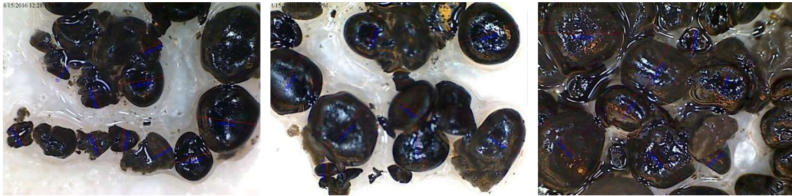
Figure 4-9. The VMS-001 USB microscope picture and the measured diameter of granules sampled from EGSB reactor with the range from 0.41 – 2.32 mm..
