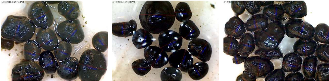
Figure 4-8. The VMS-001 USB microscope picture and the measured diameter of granules sampled of UASB – E Convert with the range from 0.6 – 2.74 mm.
