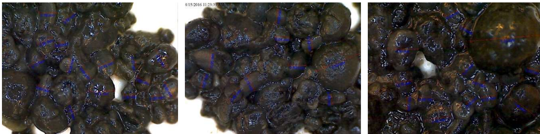
Figure 4-12. The VMS -001 USB microscope picture and the measured diameter of granules sampled from E-Convert (new) with the range from 0.2 – 3.75 mm.
