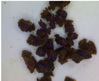
Figure 4-6. The VMS-001 USB microscope picture and the measured diameter of coffee grit 3 with the range from 0.23 – 1.23 mm.
