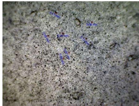
Figure 4-19. The granular size distribution of Saugbrugs (old) exited at 1.2\text{ m h}^{-1} up-flow velocity with range from 0.06 – 0.19 mm.
