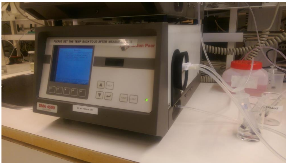
Figure 3.1: The density meter structure in operation.
