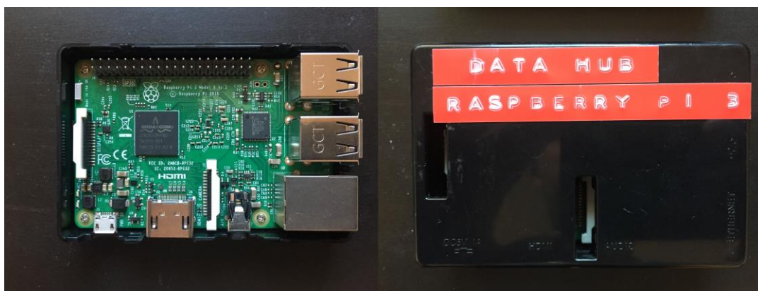
Figure 9-17 Raspberry Pi 3 data hub prototype
