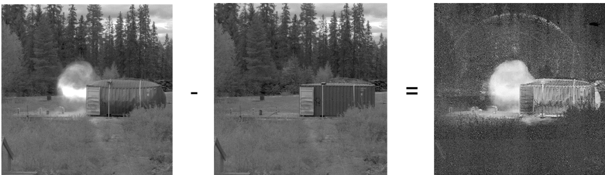
Figure 4.1 Principle of the image processing: Subtraction of an undistorted image (middle image) from a distorted image (left image) yields the result shown in the right image
