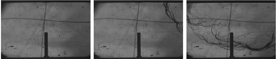
Figure 2.16 Images from schlieren test of dispersion and ignition of hydrogen in the 3 m long channel.
