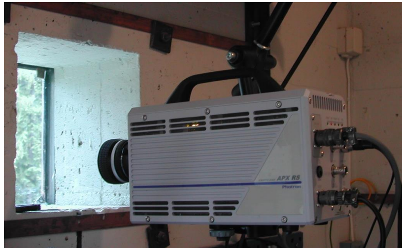
Figure 3.10 Photron APX-RS high-speed camera used in the ISO container experiments.
