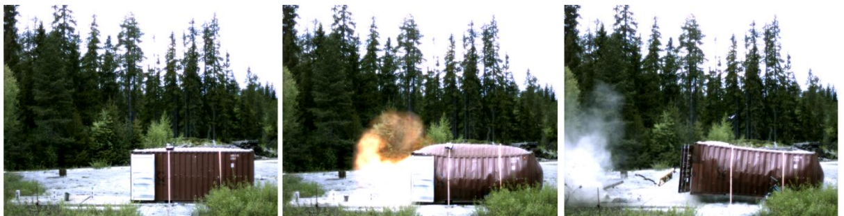
Figure 3.21 Image series of Experiment 39, captured by the Photron FASTCAM-APX 120KC colour high-speed camera. The images were captured with a frame rate of 500 fps; the time between the middle frame and the right frame is 36 ms.
