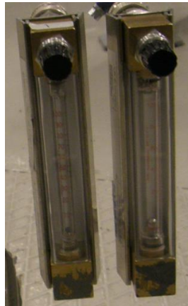
Figure 2.3 F&P Purgemaster flow meter.
