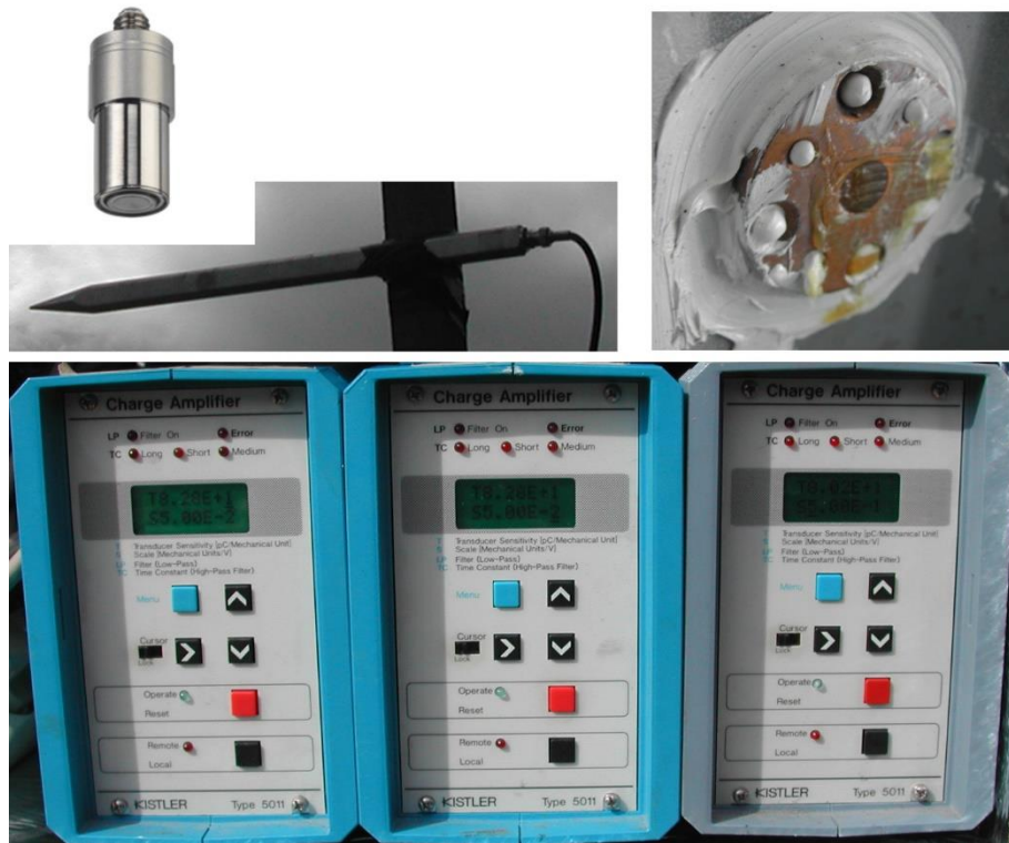
Figure 3.7 Instrumentation for pressure measurements. Top left: Kistler 7001, top right: Kistler 7001 mounted in brass plate in container wall, top middle: LC-33 pencil shaped transducer mounted on a pole located outside of the container. Bottom: Kistler charge amplifiers.
