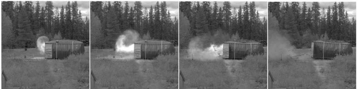
Figure 3.23 High-speed images from experiment 39, at time steps 153, 166, 190 and 253 ms, counted from camera trigger time.
