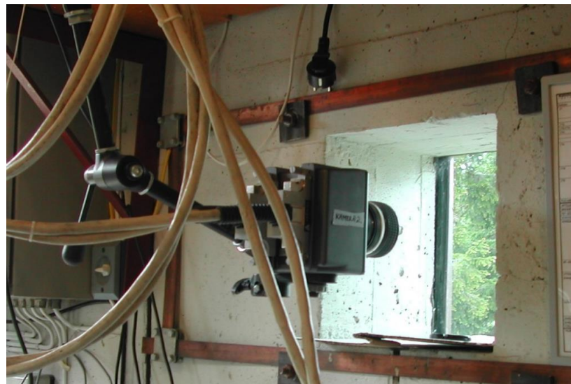
Figure 3.11 Photron FASTCAM-APX 120KC colour high-speed camera used in the ISO container experiments.
