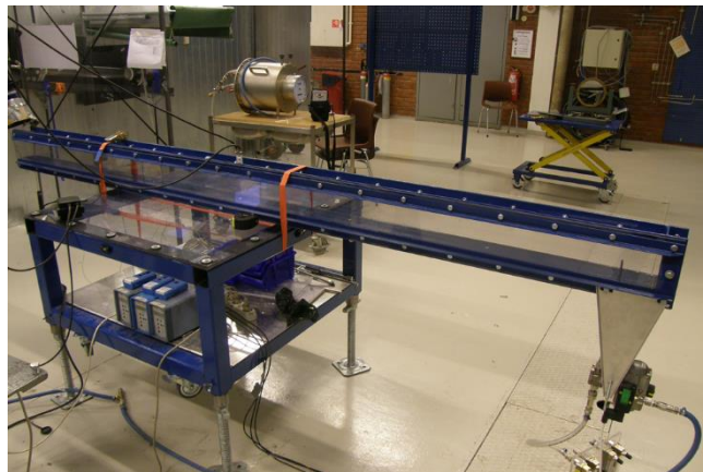
Figure 2.1 Experimental setup of the 3 m long channel.
